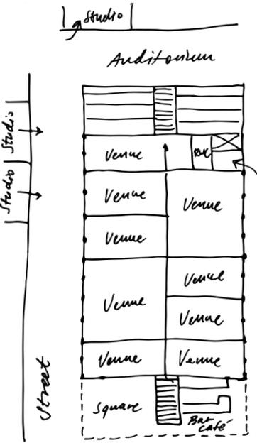
Figure 69. The sketch above is from the final stages of the design process, where the addition developed into the design it has today. Another staircase is added, and the back space is more efficiently used and holds one studio.
