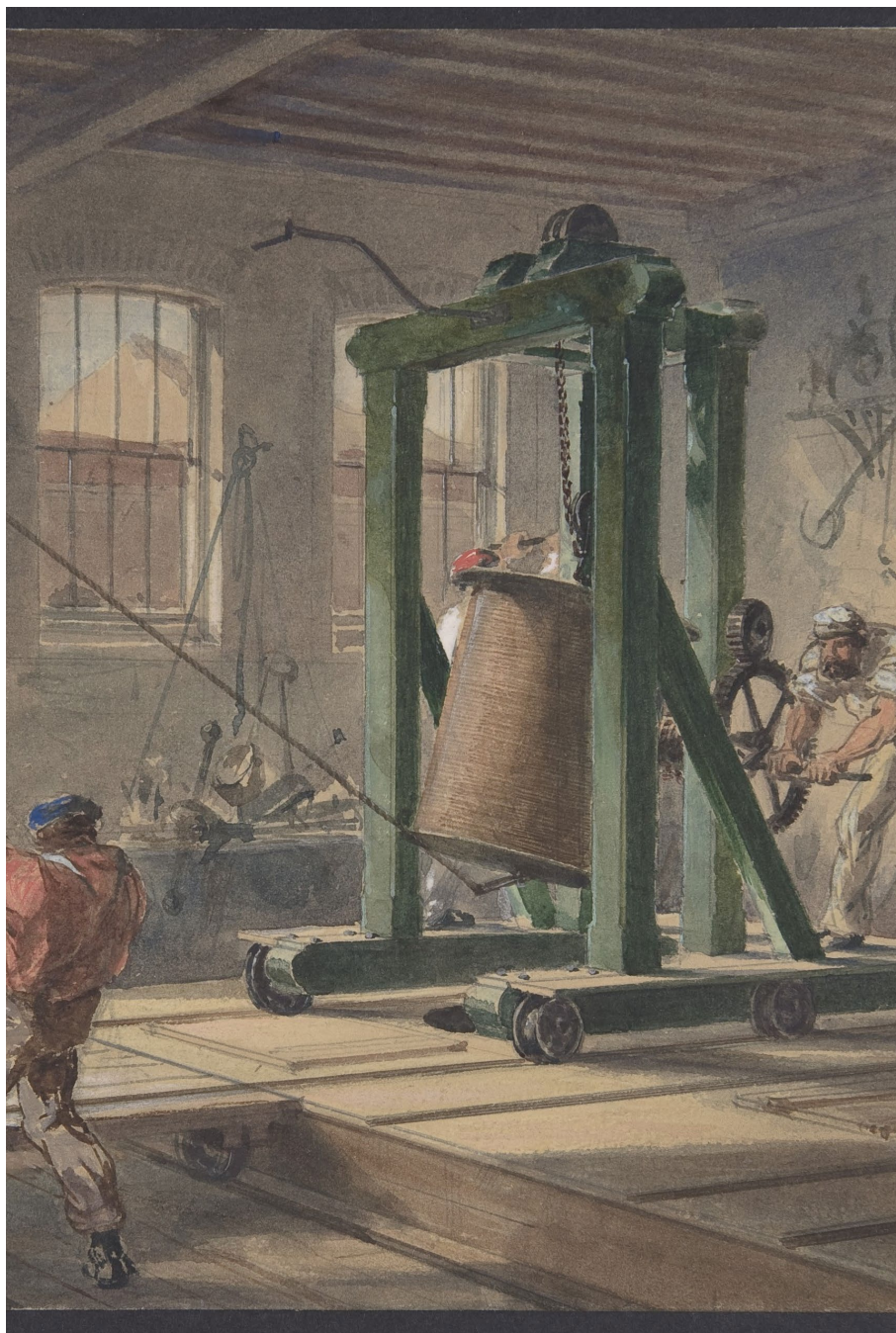
The Reels of Gutta-percha Covered Conducting Wire Conveyed into Tanks at the Works of the Telegraph Construction and Maintenance Company, at Greenwich (1865).
