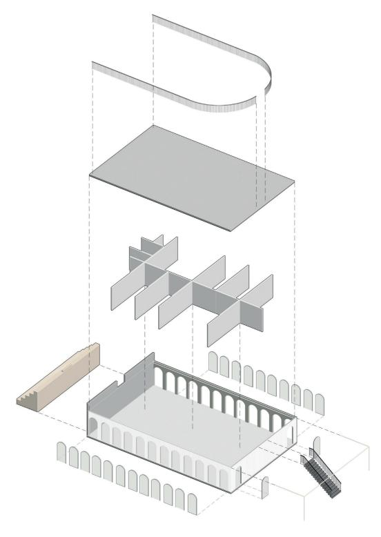
Figure 62. Axonometric diagram which shows the different parts of the addition.
