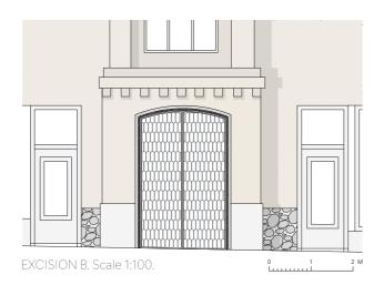
The elevation above shows the southern facade from Södra Larmgatan. This entrance has two layers, one gate and one entrance to Artilleristallarna. The gate (above) is open during the day, and closed during night. The gates consists of iron work and are created by a local blacksmith. The pattern relates the arched shape which occurs inside.
