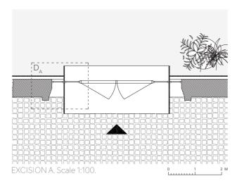
Above, the drawing shows the entrance towards Magasinsgatan. It it characterized by its dark grey, welded metal sheet portal. It offsets from the original opening to counterbalance the shape of the original gate. It is complemented with glazed double doors and windows. This approach is implemented for the southern entrance as well. When walking through the entrance portal, the angle of vision is narrowed down to increase the unveiling and experience of the great hall.
