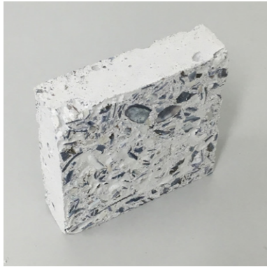
Bigger shells, visible after sanding.
