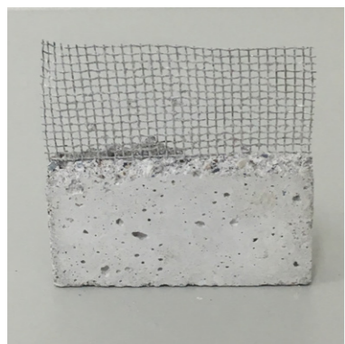
Mesh visible through splitting element.
