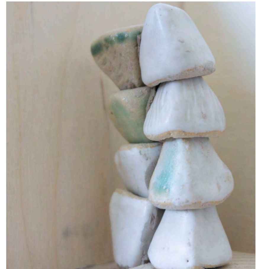
Test-pieces of bricks in burnt and glazed clay, scale 1:10, with soft clay (mortal) as a way to connect them
