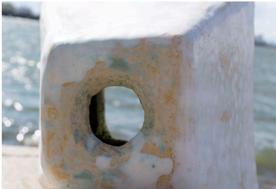
Pictures of 1:1 prototype of the brick, to give an understanding and sensation of what the brick may look like in actual scale. Different textures of the sides of the brick have been tested and the idea of having another glaze on the inside have been kept.
