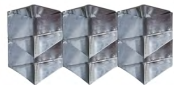
Fig. 4.19 – Upcycling of used air duct - cutting angle and folding
