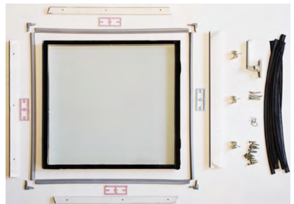
Fig. 4.33 – Demounted windows from a demolition , Own photo
