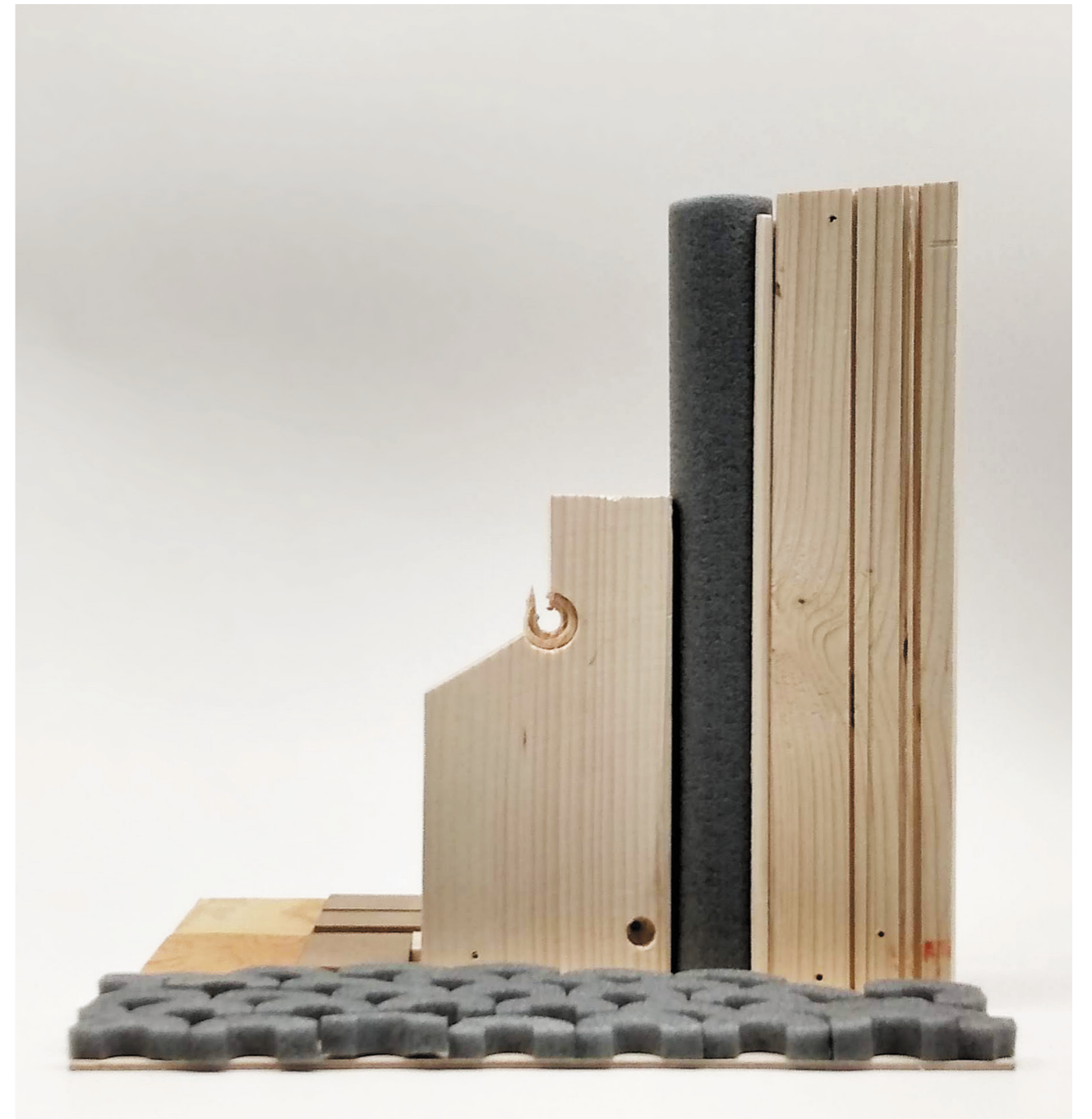
A floor is made from cut pieces of the plastic tube. A wall is made from tubes and a wood piece.
