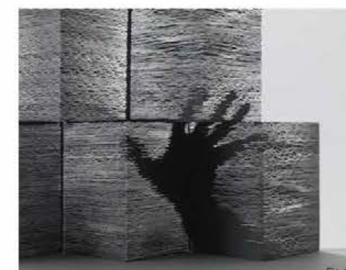
Fig. 15 Material: Translucent concrete panel
