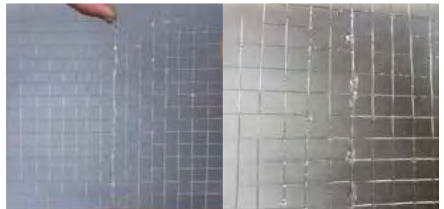
Fishing net 150x150mm, mesh 10x10mm, wire Ø 0,25mm. The water fell down only where you poured it. The larger mesh did not allow multiple ways down. Droplets did form after a pourdown since the mesh could not absorb.
