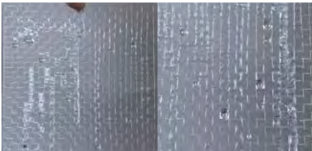
Fishing net 150x150mm, mesh 5x5mm, wire Ø 0,25mm. The water chose different ways down depending where you poured it. The smaller mesh allowed multiple ways. A lot of droplets formed since the mesh could not absorb.
