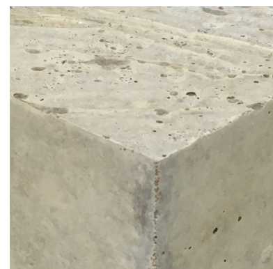
Concrete mixture using sand vs crushed mussel
