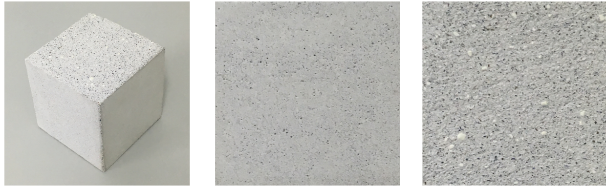
Sanded surfaces with different roughness
