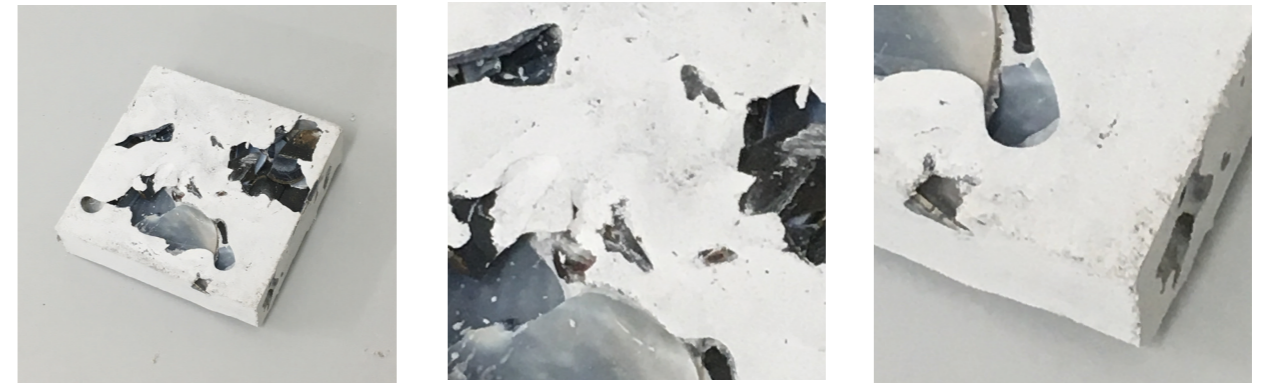
Before: Uncrushed shells were placed in the mold, the result was uncontrolled holes in the cast
