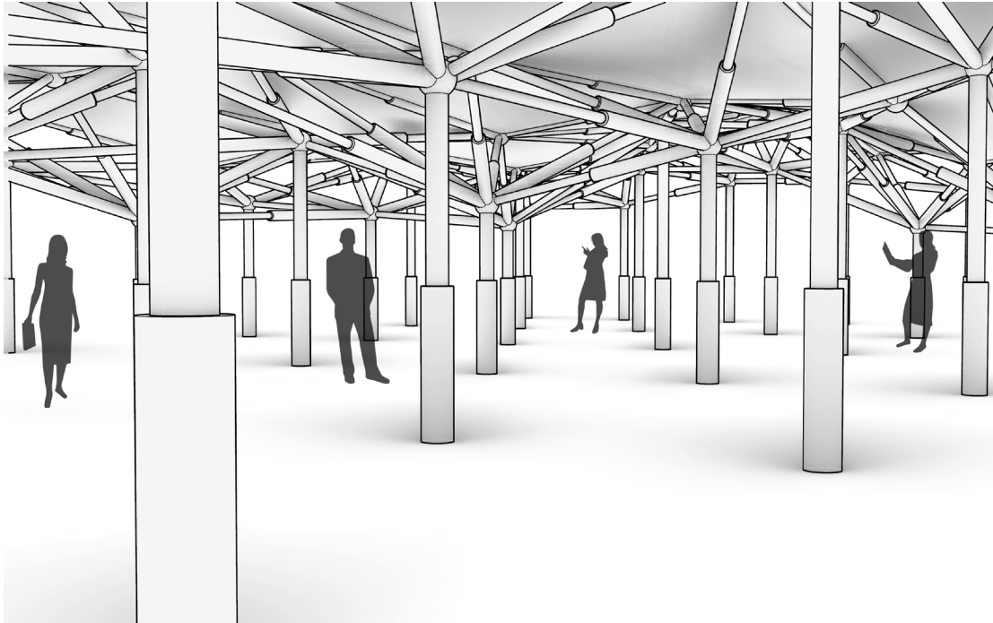
Phase 1. Kinetic Space Frame. Perspective from underneath the system, showing the kinetic columns carrying the system.
