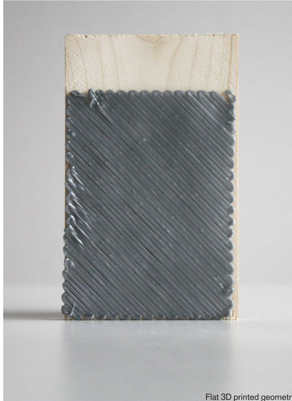
3D printed bulb fixes print onto wooden piece
