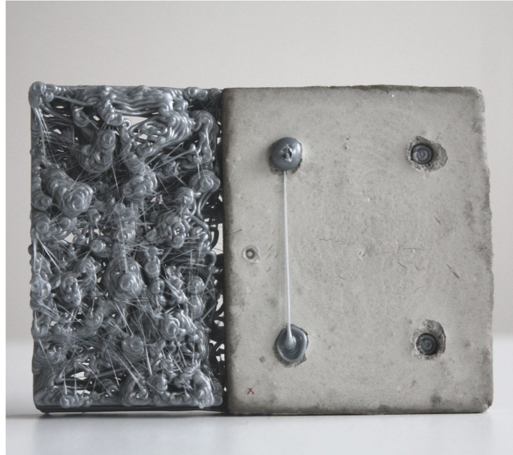
New filament remelted the 3D printed plugs
