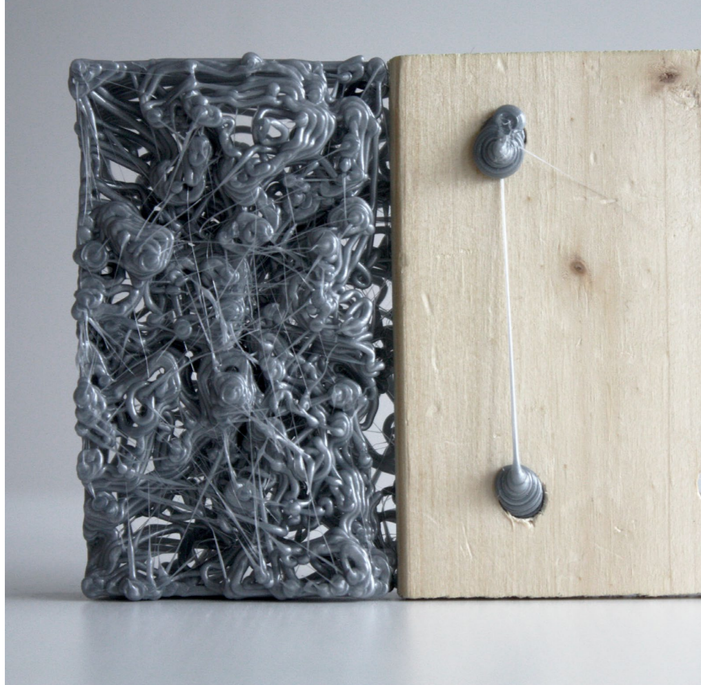
3D printed geometry reaches behind wooden object
