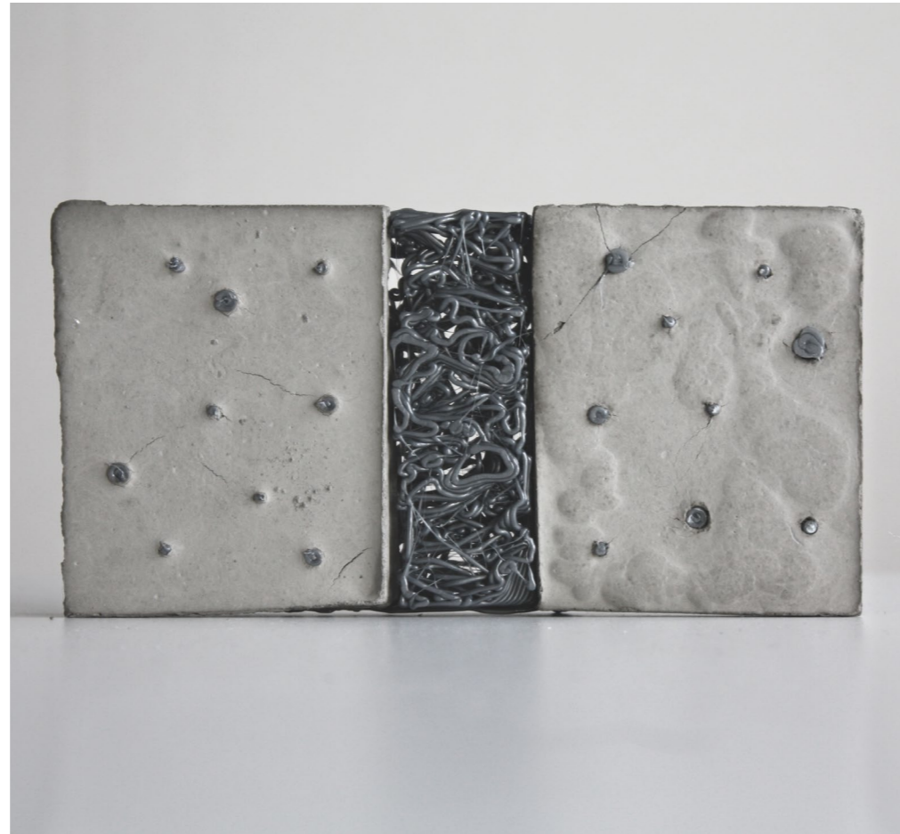
3D printed geometry fills in the gap in between concrete blocks
