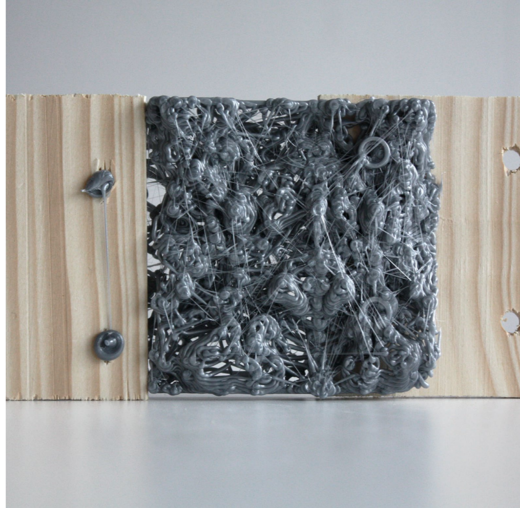
Single piece of 3D printed geometry is able to hold 2 wooden blocks together
