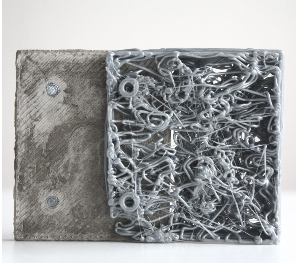
3D printed plugs were left into the concrete block
