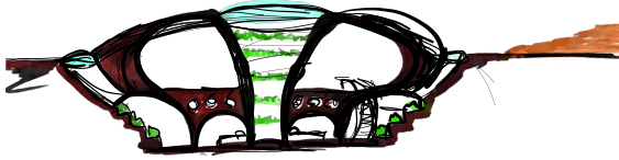
Early sketch where the habitat was built underground. Light channels were dug down to a subsurface garden in the corridor surrounding the bedrooms
