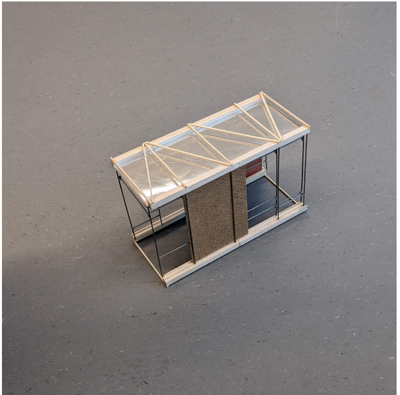
Scale model of a scaffolding unit, with frames that allow flexibility to slide in and out different materials on the four planes of the sidewalk room 4 .
