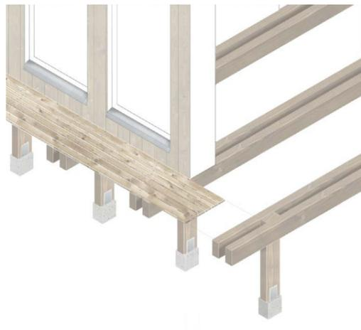
Plinth-foundations have a low impact on the landscape and surroundings. Adjustable to many different conditions. Keeps the terrain passable for insects, plants and small animals. Footbridges makes human passing more comfortable without leaving imprint on the ground. Accessibility around the facade makes it easier to maintain and creates an outdoor passage.
