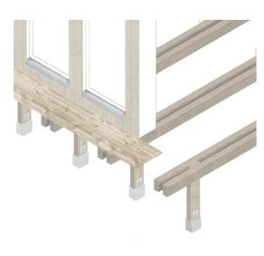
Plinth-foundations have a low impact on the landscape and surroundings. Adjustable to many different conditions. Keeps the terrain passable for insects, plants and small animals. Footbridges makes human passing more comfortable without leaving imprint on the ground. Accessibility around the facade makes it easier to maintain and creates an outdoor passage.
