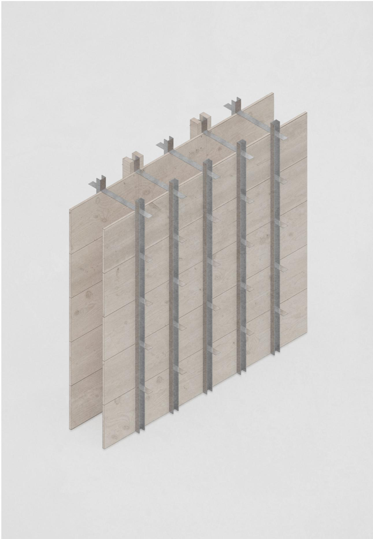
The load-bearing walls are constructed using a rather primitive in-situ cast concrete method that has been promoted through projects by architects such as Luigi Snozzi and Peter Märkli. The method is unconventional but gives full control of all visible surfaces. Iron-oxide pigments are mixed into the cement mix to create a colour nuance similar to the surrounding landscape.
