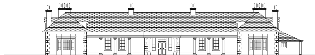
Drawn example 1c: Boleskine House, original courtyard elevation 1:300. Windows in grey have Georgian proportions.
