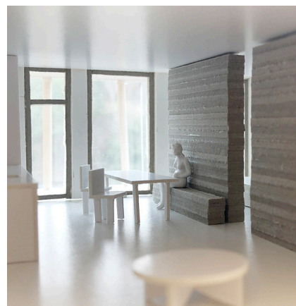
Sketch model of apartment 1:50, the heat walls gives warmth, thermal inertia and works as a spatial divider of the apartment.
