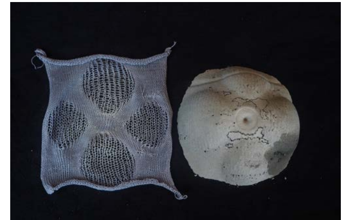
#9 Drop stitch, medium thick yarn, concrete with nylon membrane
