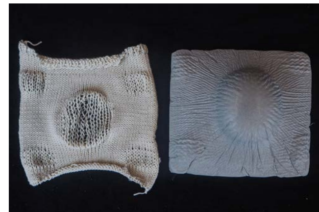
#10 Drop stitch, medium thick yarn, concrete with plastic membrane
