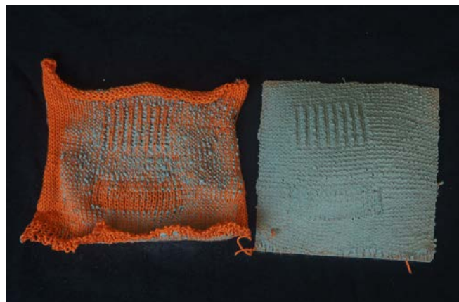
#6 Rib knitted combined with tight knit, cotton yarn, concrete
