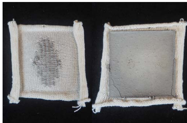
#4 Combined loose and tight knit, cotton yarn, concrete
