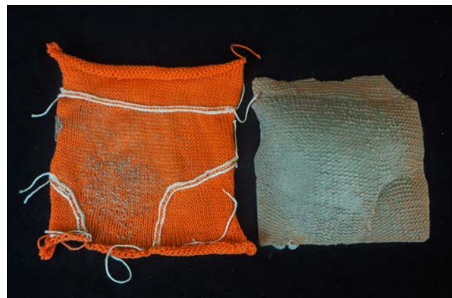
#7 Tight knit with stiffeners, cotton yarn, concrete
