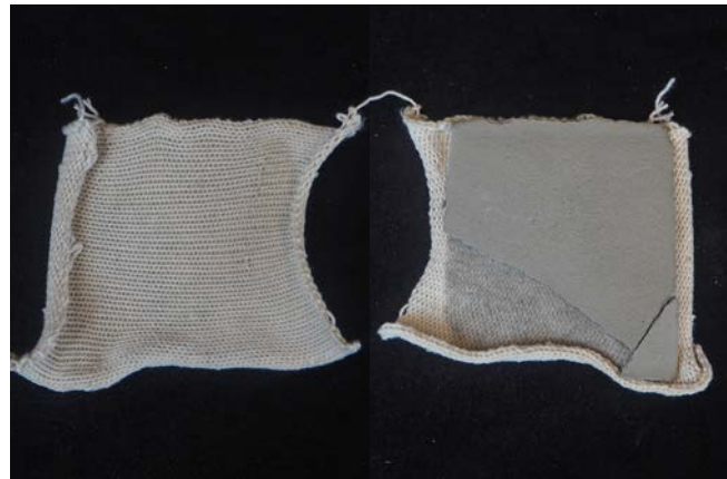
#1 Tight knit, cotton yarn, concrete
