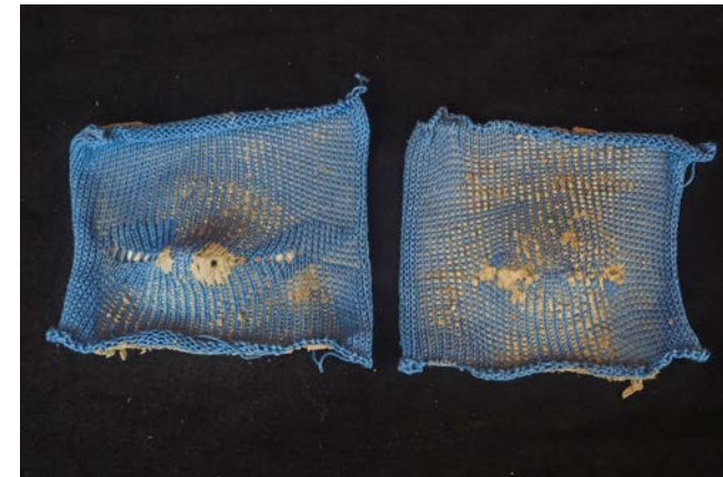
#8 Short row, medium thick yarn, concrete
