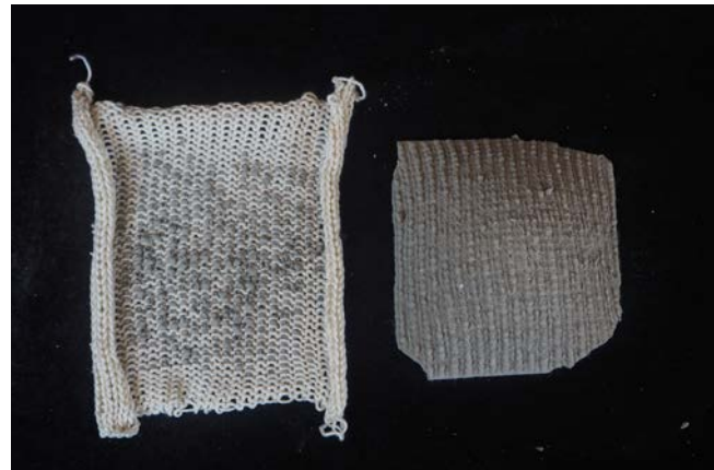
#2 Loose knit, cotton yarn, concrete
