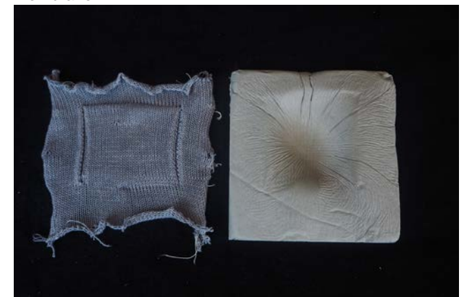
#11 Integrated pocket with inflated balloon, thin cotton yarn, concrete with plastic membrane
