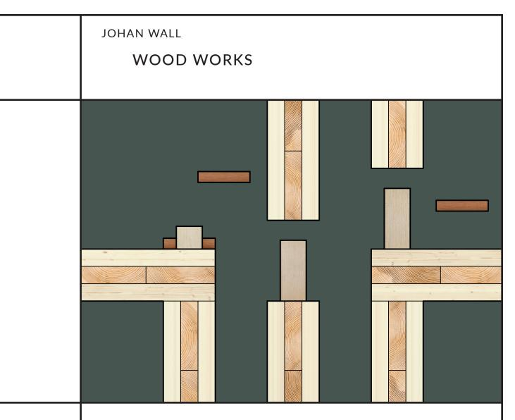
innovative An system of wood connections, originating in state-of-the art circular design principles and traditional joinery craftsmanship, is developed for a structural system of engineered wood products. The joinery system is an architectural exploration aimed at demonstrating how timber structures could be assembled to facilitate easier deconstruction and increase the reuse potential of structural components.
