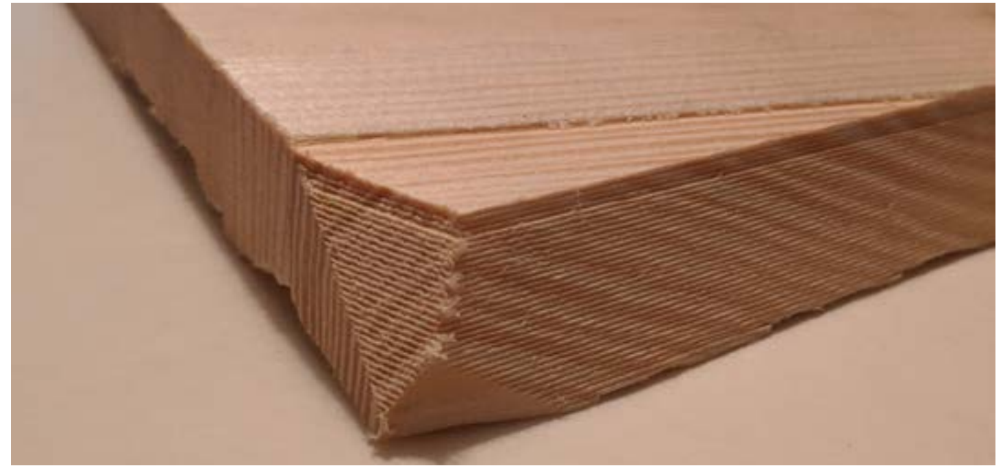
A macro photo of the ridges left by the approximation of an angled surface by a straight endmill.
