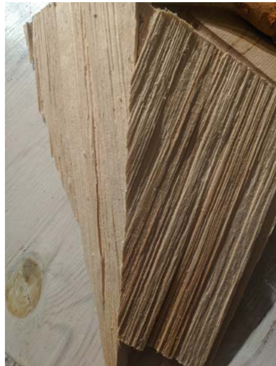
When the pieces are placed together the intended texture is finally revealed. The angle of which each piece was milled greatly influences the visual texture.
