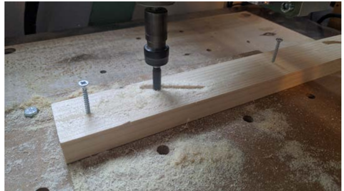
Above: CNC router that is used for physical testing Below: The actual routing of a pocket for a
