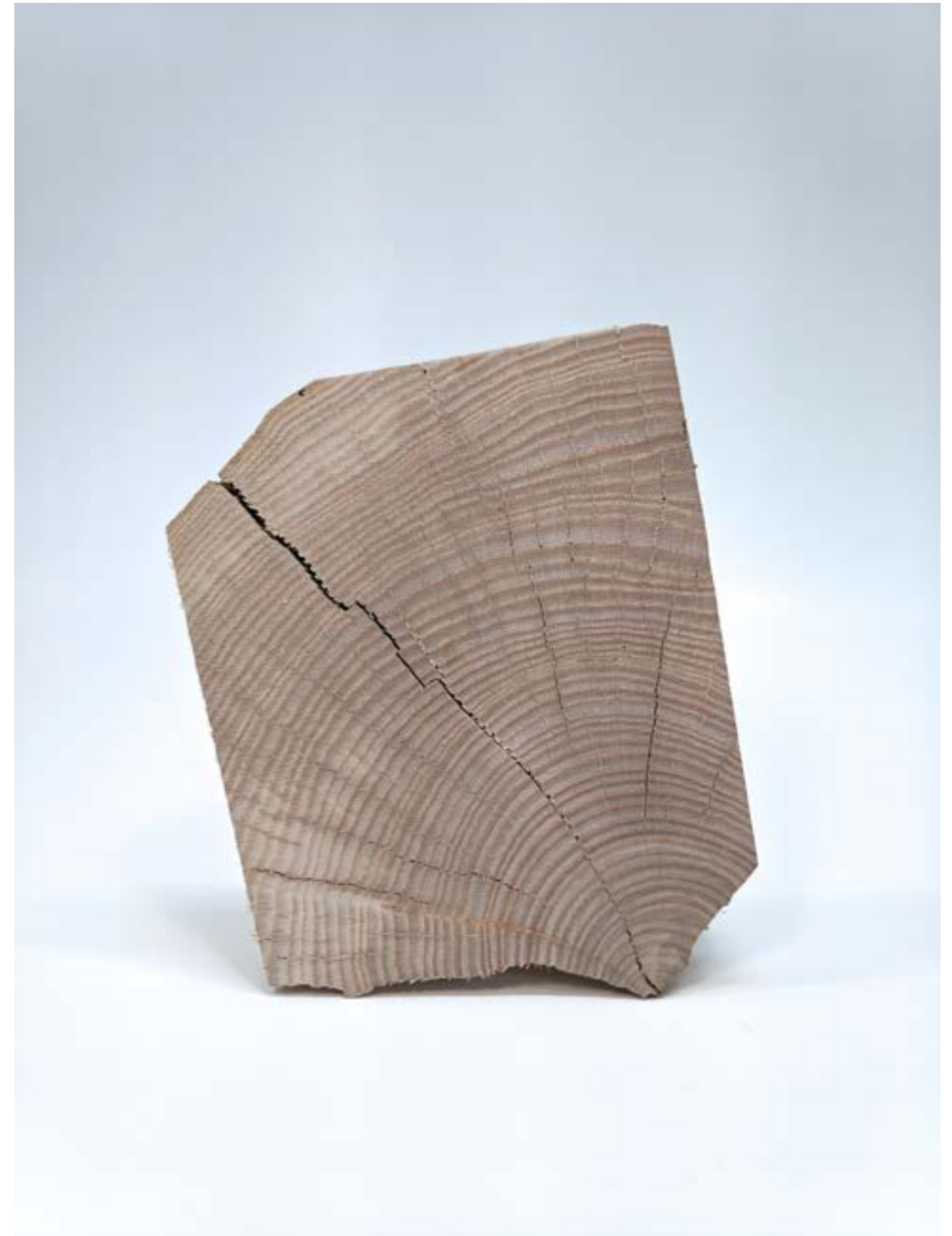
A slice of walnut timber, showing a crack propagate through the piece. The shape and direction is based on the grain structure formed when the tree grew, but also allows for a non linear split due to irregularities of a natural material.
