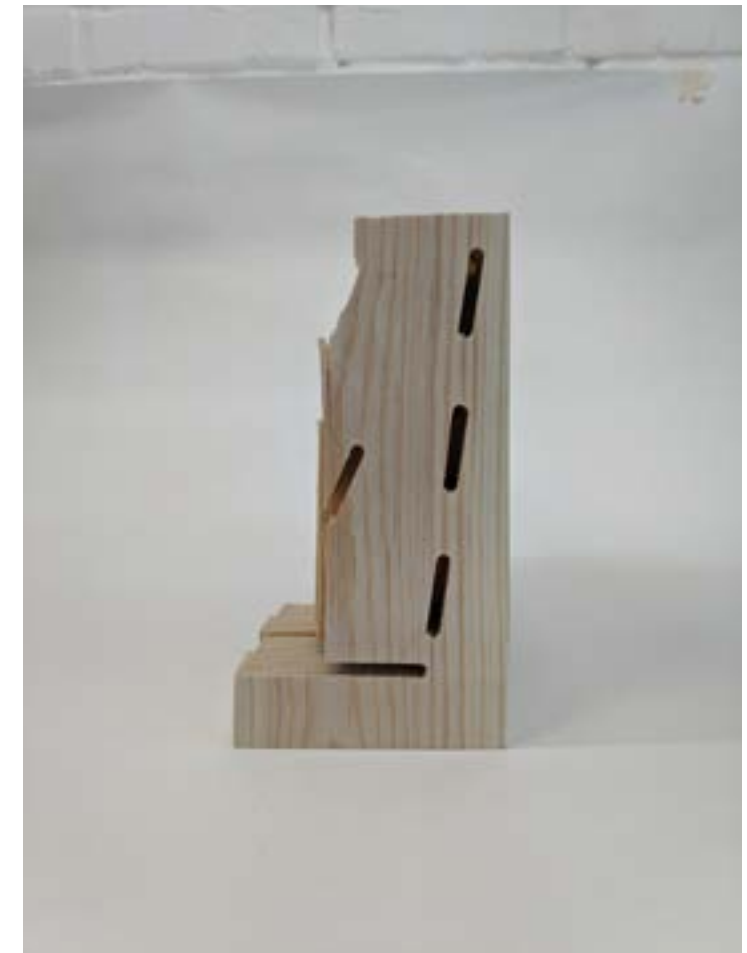
Issue of failure to cleave becoming apparent.
