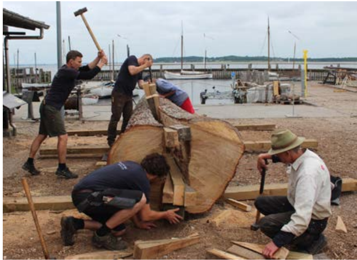
Cleaving of wood for boat building
