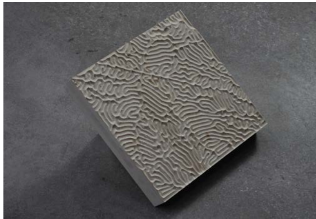
Milled piece CLT 1:2 350x350x65 Milling time: 5 min
