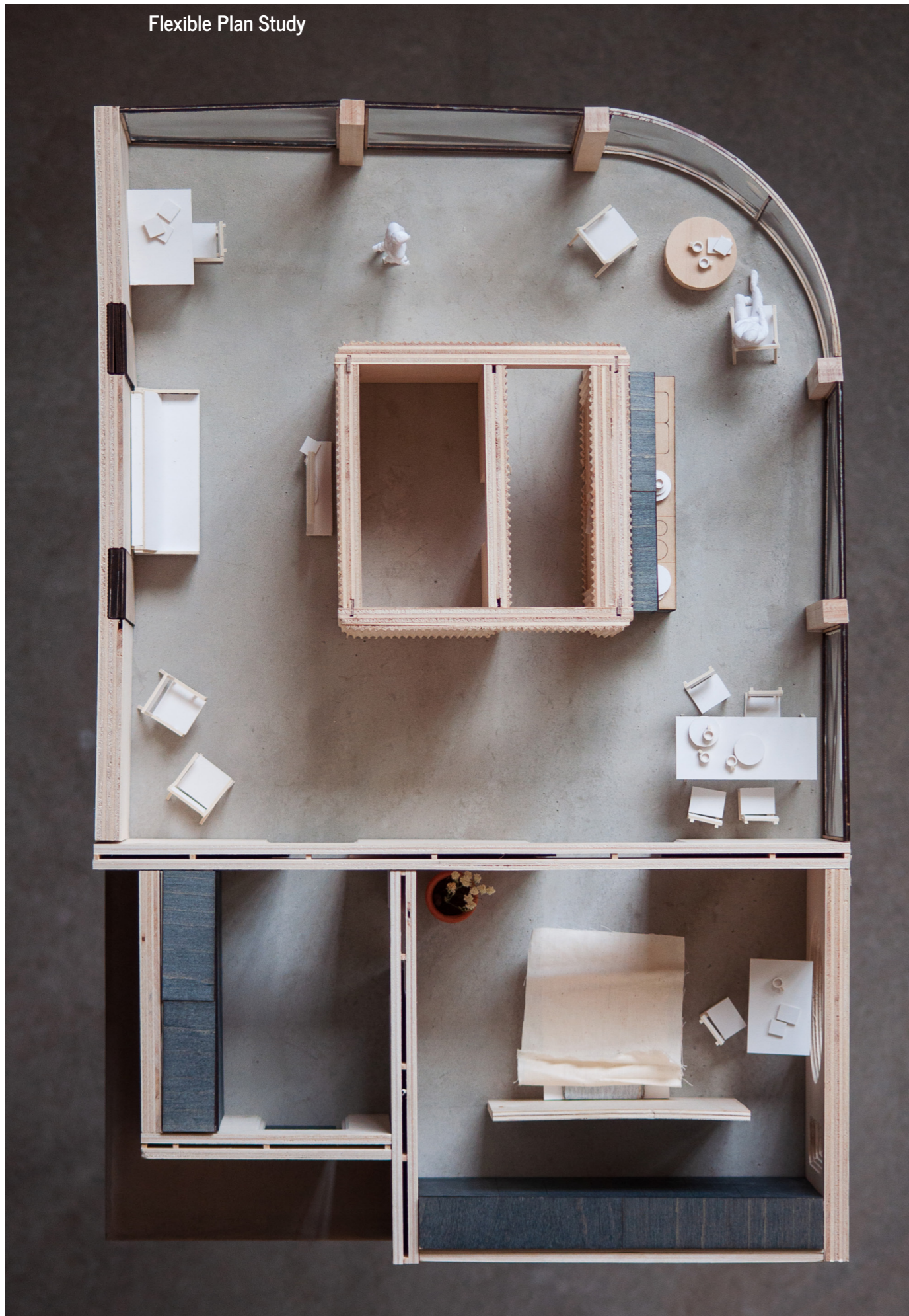
The apartments have an open plan around the core which holds facilities like wet surfaces, shafts and plumbing. The plan is flexible with the possibilities to
