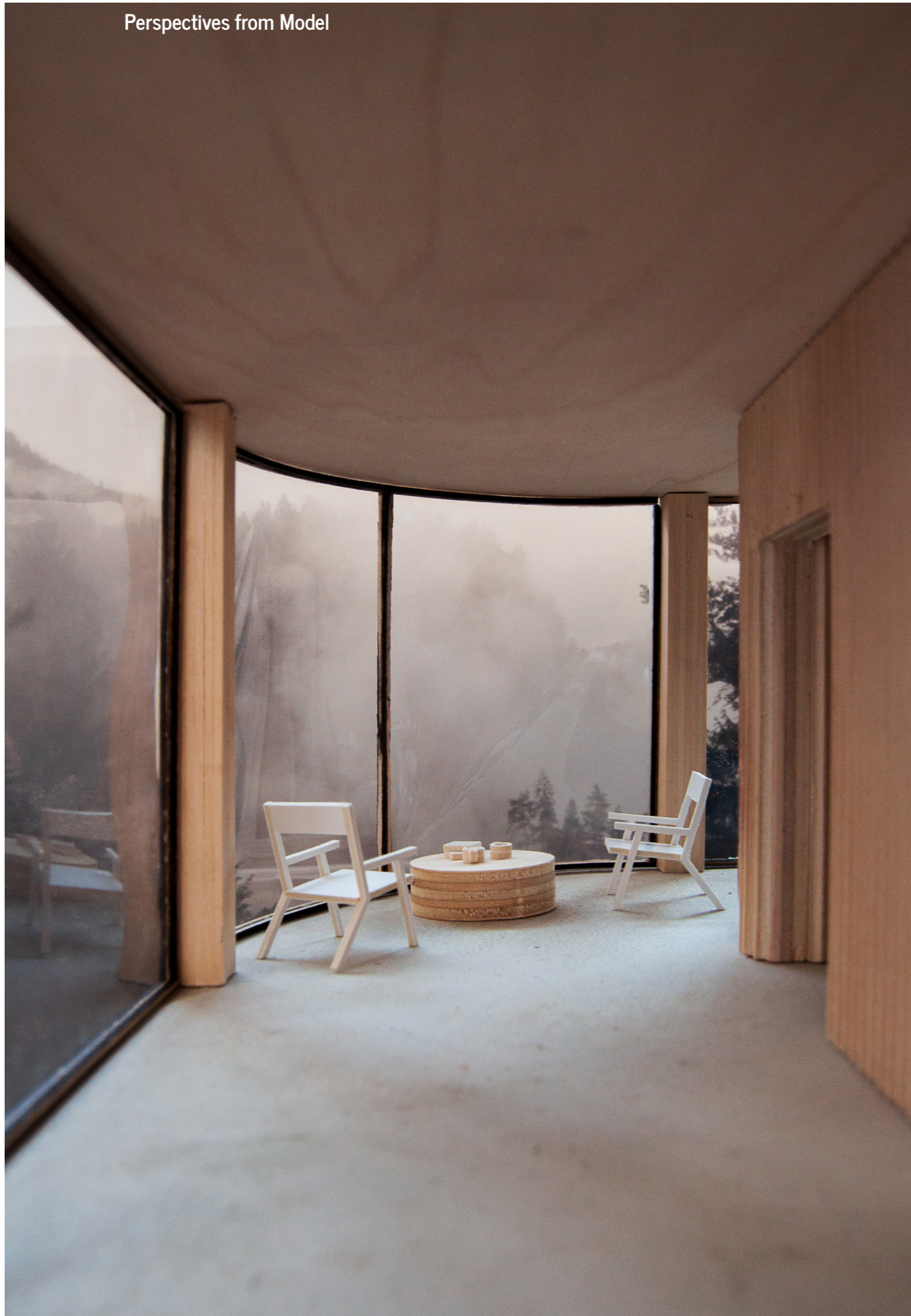
Interior view of the rounded slab and window, the rounded corner limits the wind loads
