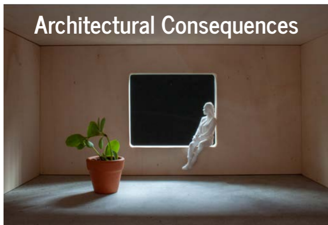
Model Photos Row 1: Perforations can without any major added costs be ornamented with the help of a CNC-mill.
