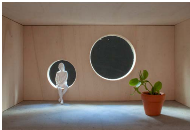
Model Photos Row 3: Perforations are not restricted to be shaped in an orthogonal way when made with a CNC-mill. The round shape of the milling
