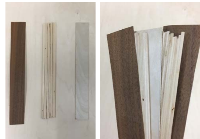
Combination of wooden materials to cater technical specifications in Glulam models. Different kinds of wood are usually combined in furniture making.
