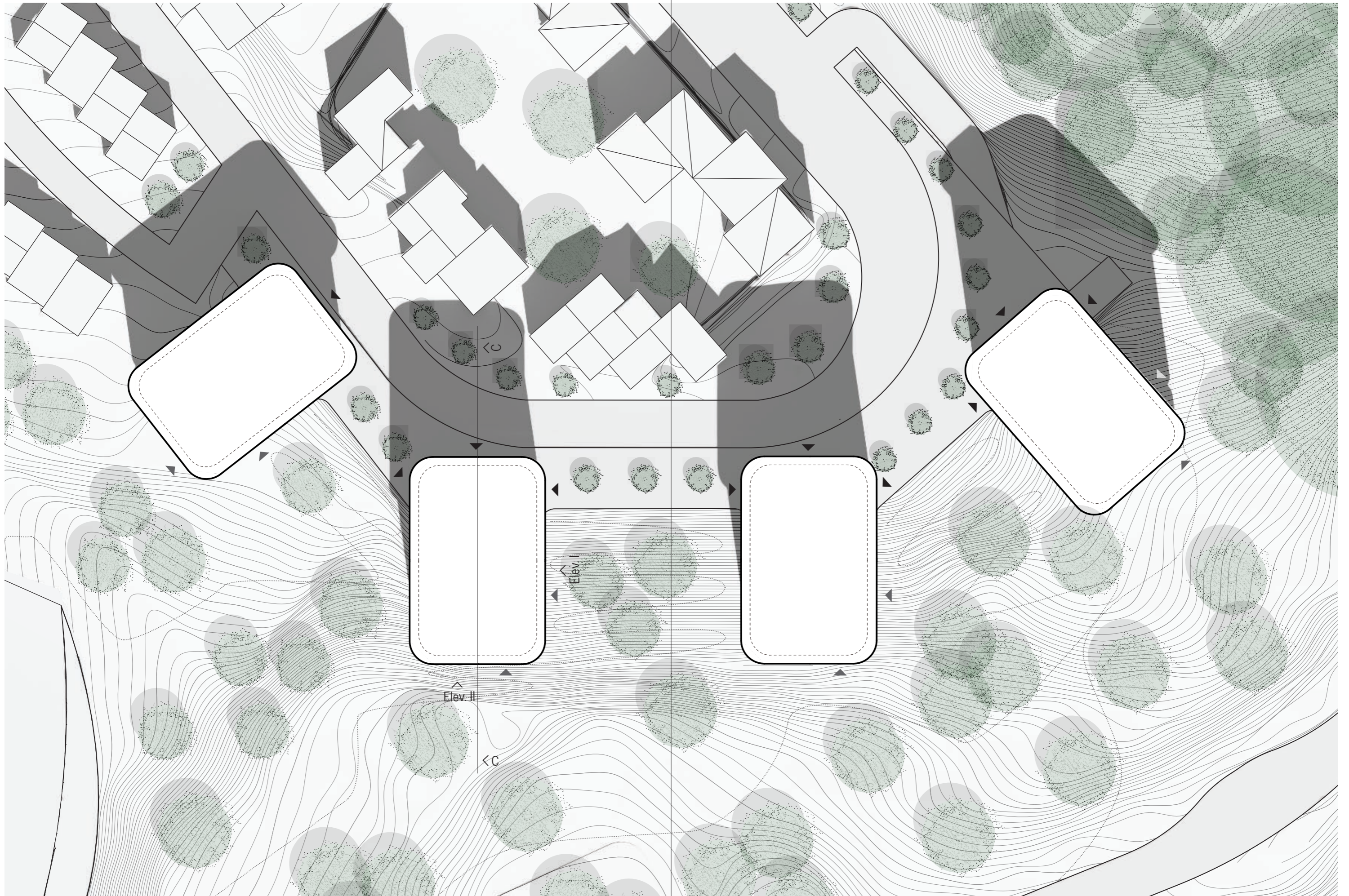
Site Plan Plan 1:500 Sun/shadow condition 12:00 - 21 June
