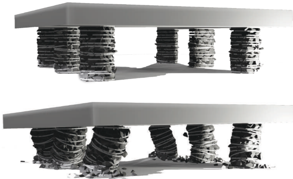
Early simulation trying to test the load-bearing capacity of an aggregated structure
