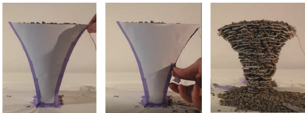
When the structure was completed, the paper mould was removed to reveal the finished aggregated model
