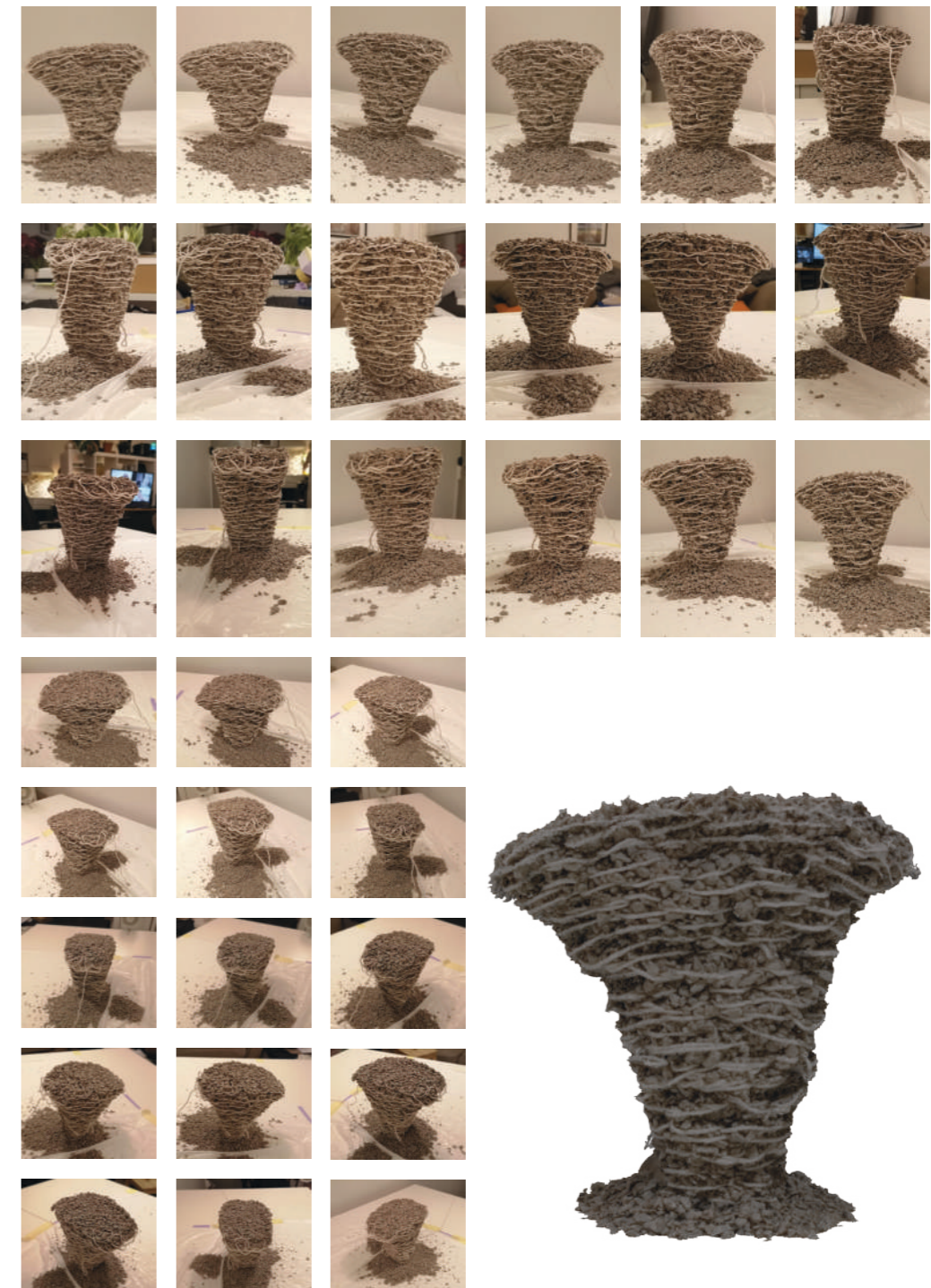
The photos were used to create the 3D-model on the right
