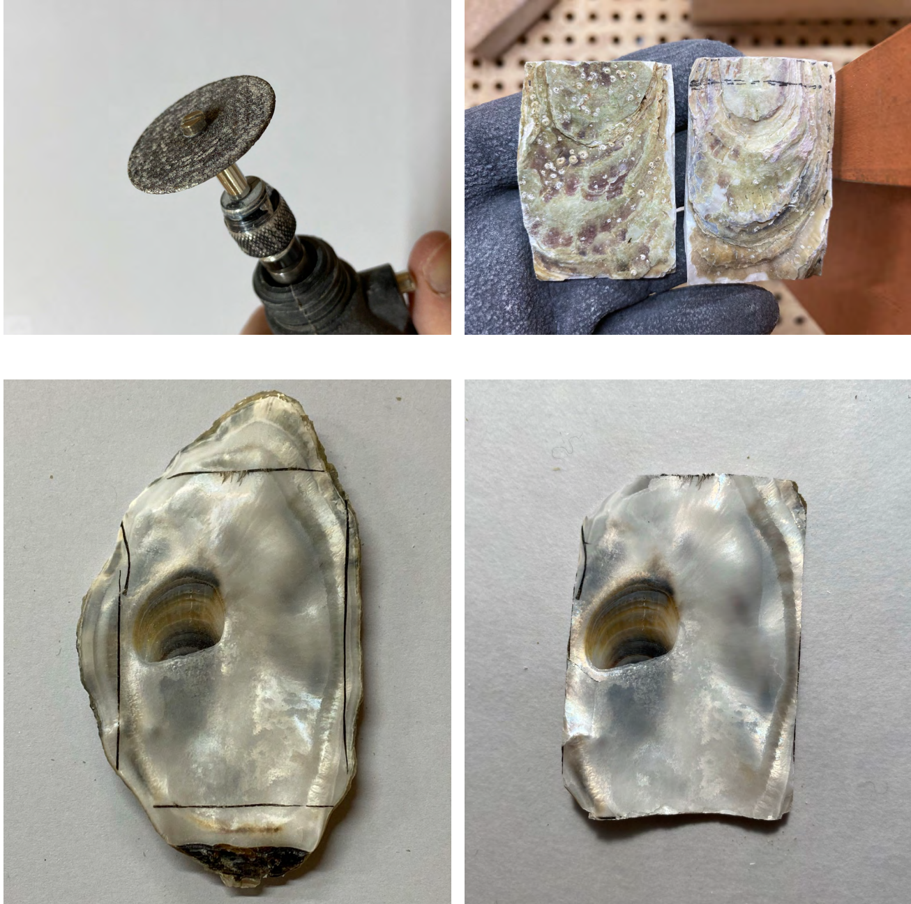
Cutting oyster shells: 3.5cm*5.5cm
