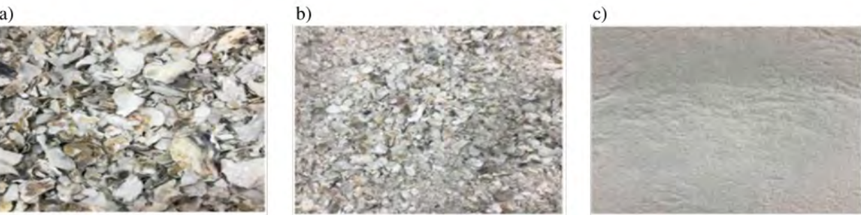
Fig. 2. (a) Surface of oyster shell, (b) Crushed oyster shell, (c) Powdered shell using electric furnace about 1000 °C
