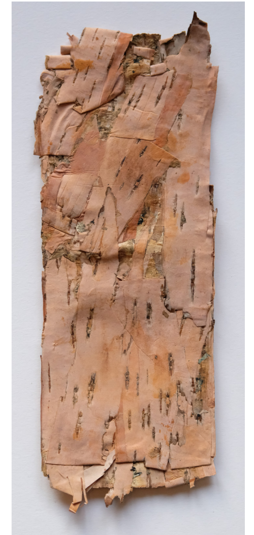
The left over material from the turning and sculpting experiments was packed in metal cooking forms, filled with water, pressed and heated in an oven at 100°C for thirty minutes.
