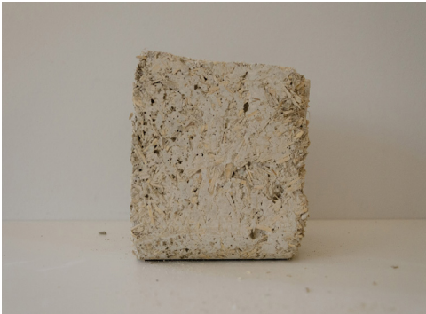
Image 49. Hemp-lime sample made during workshop at RISE. Its mass ratio (shiv:binder) is (1 shiv: 2 binder). The lime binder used is from Tradical.
