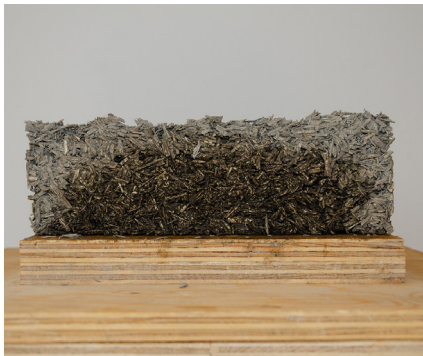
After 3 days, the corners are dried out. The surface while drying is quite fragile and brittle. Pieces can come of if handled without care.
