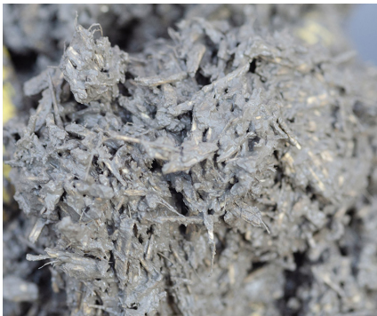
Zoom on hemp-clay mix, the mixture is rather sticky because of the clay-slip.
