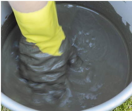
First mixing clay and water together. The mixing was done by hand, in small amounts. It is a rather intensive procedure, using a paddle mixer would be advisable.
