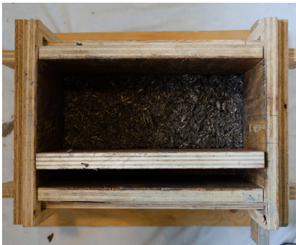
Putting the hemp-clay mixture in the mould, layer by layer, and tamping everytime to remove air gaps.
