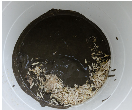
The clay-slip was prepared before-hand and used only several weeks after. It was still perfectly workable after stirring the slip. This slip is the same as the viscosity test on the previous page. 1 volume of slip is mixed with 2,5 volumes of hemp shiv.
