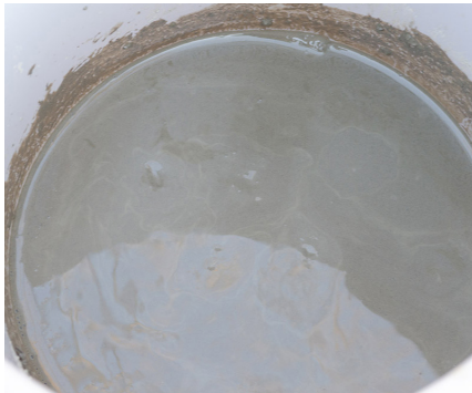
Zoom on clay-slip. This was a thick slip of proportions 4:1 (clay:water).
