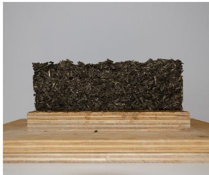
The sample can be demolded immediatly. It is left to dry.
