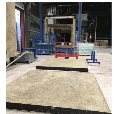
Finished panels. Left to dry for a week before put vertically.
