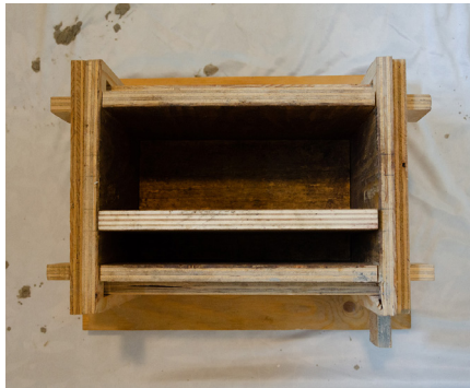
Wooden mould used to make the sample.
