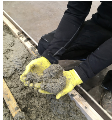
Testing the mixture: A small ball of hempcrete breaks in the middle.
