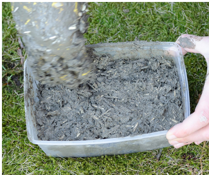
Mold the hemp-clay into a form. The sample can be demolded immediatly and left to dry.
