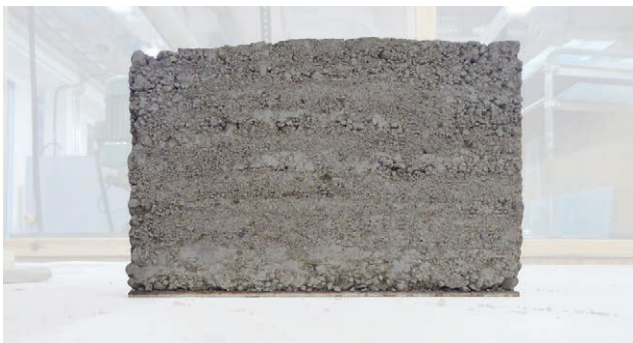
Figure 23. Mixture 1, too dry mixture, due to misunderstanding recommended water content. Ball drop test not possible. 1:10 relation of water and rammed earth mix. Rammed sample is very fragile.
