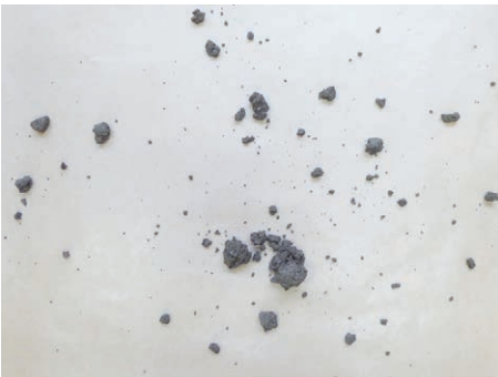
Figure 24. Mixture 2. More water was added to the original mix. Falling into pieces in ball drop test. 1:7 relation of water and rammed earth mix. More compact result with a better looking surface finishing.
