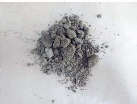
Figure 23. Mixture 1, too dry mixture, due to misunderstanding recommended water content. Ball drop test not possible. 1:10 relation of water and rammed earth mix. Rammed sample is very fragile.
