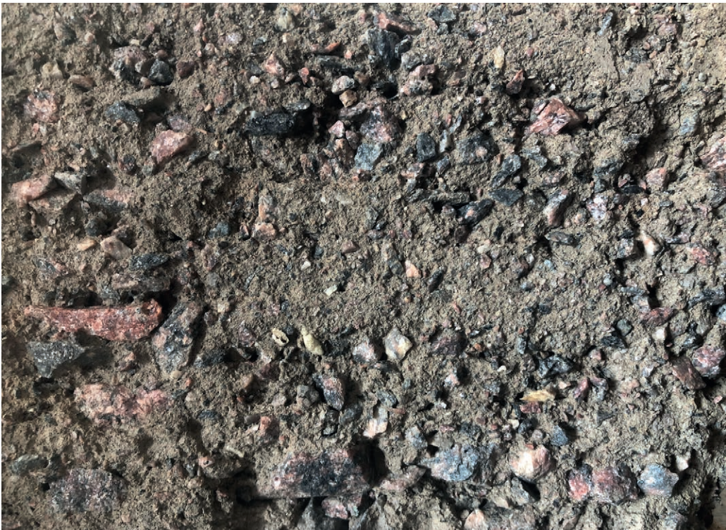
Figure 32. Mixture 2, surface after erosion test.
