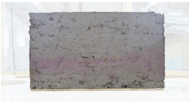
Figure 25. Mixture 3. More water was added to the original mix. Cracks in ball drop test. 1:5 relation of water and rammed earth mix. More elastic mix, hard to make compact when ramming.
