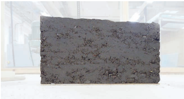
Figure 24. Mixture 2. More water was added to the original mix. Falling into pieces in ball drop test. 1:7 relation of water and rammed earth mix. More compact result with a better looking surface finishing.
