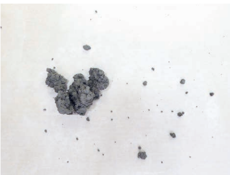
Figure 25. Mixture 3. More water was added to the original mix. Cracks in ball drop test. 1:5 relation of water and rammed earth mix. More elastic mix, hard to make compact when ramming.
