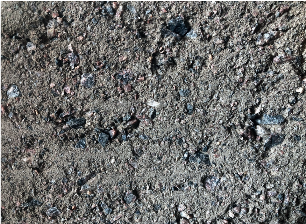
Figure 33. Mixture 3, surface after erosion test.
