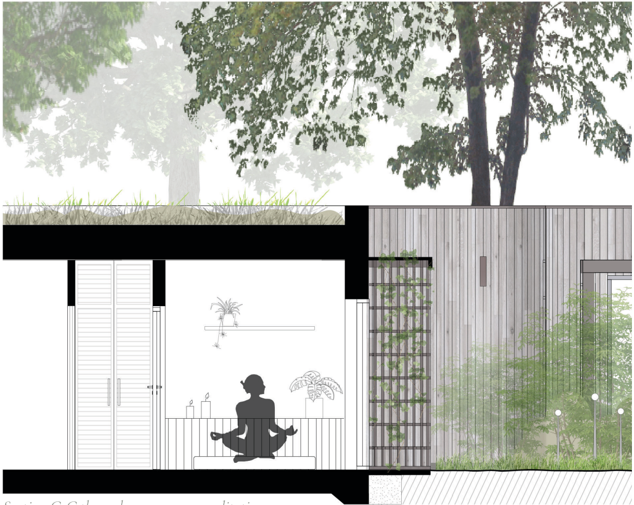
Section C-C through prep-room, meditation space and the small terrace extension framed by wooden slats with climbing plants
