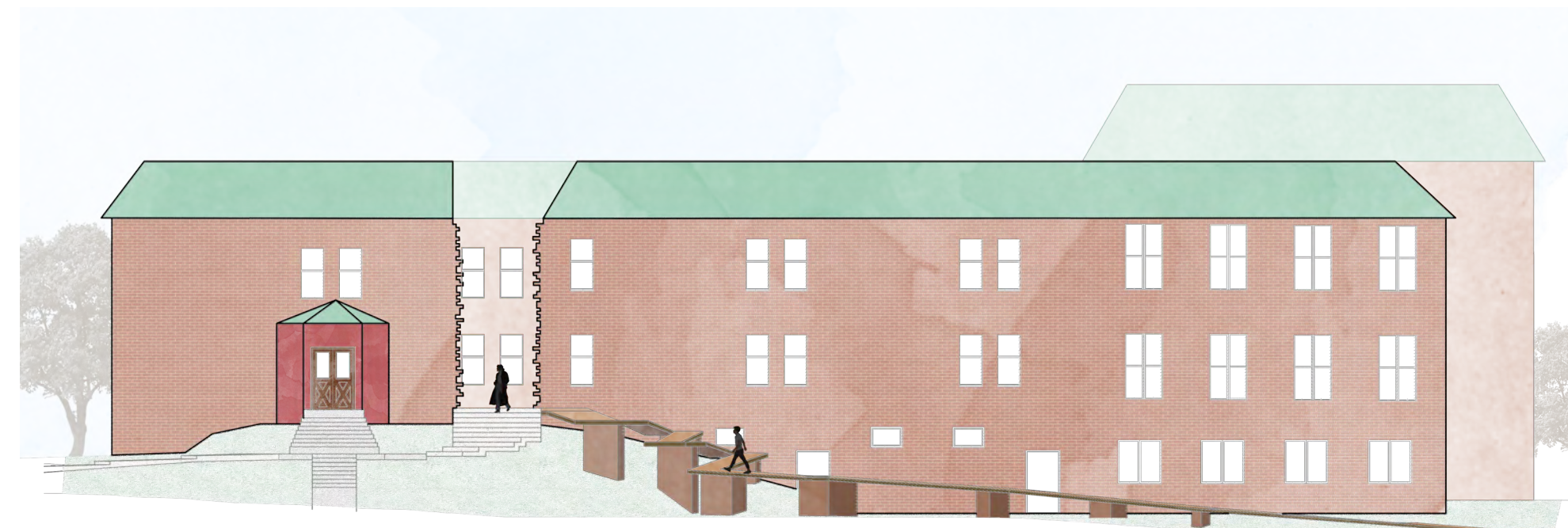
Full height opening to guide the pedestrian to the courtyard. This space is more open to correspond to the more active atmosphere of that part.
