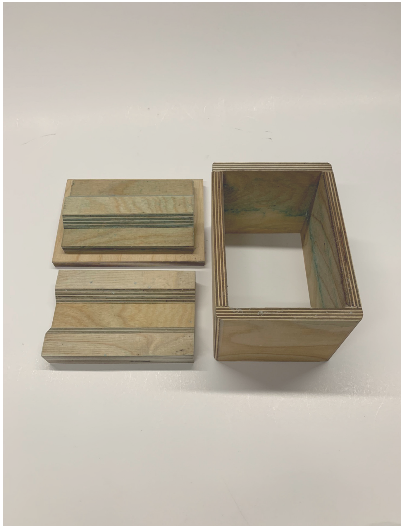
Block wooden mold
