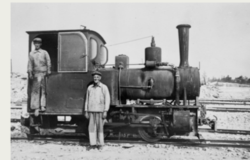
Fig 10. Photograph from the archive of the Swedish Railway Museum with the description "An Orenstein & Koppel made steam locomotive at Smöjen Limestone Quarry so either Smöjen Limestone Quarry 4 or 5 with staff."
