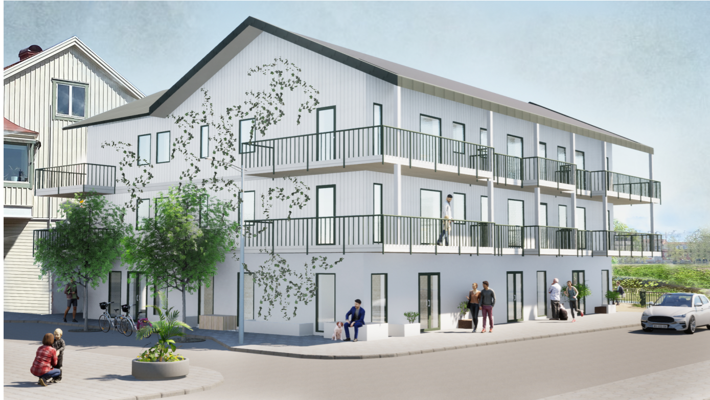
Figure 1: Perspective from the southwest. The building is shaded by trees and ivy to the west. Balconies and roof eaves shade the building in summer and prevent overheating. Along the promenade you enter the restaurant.
