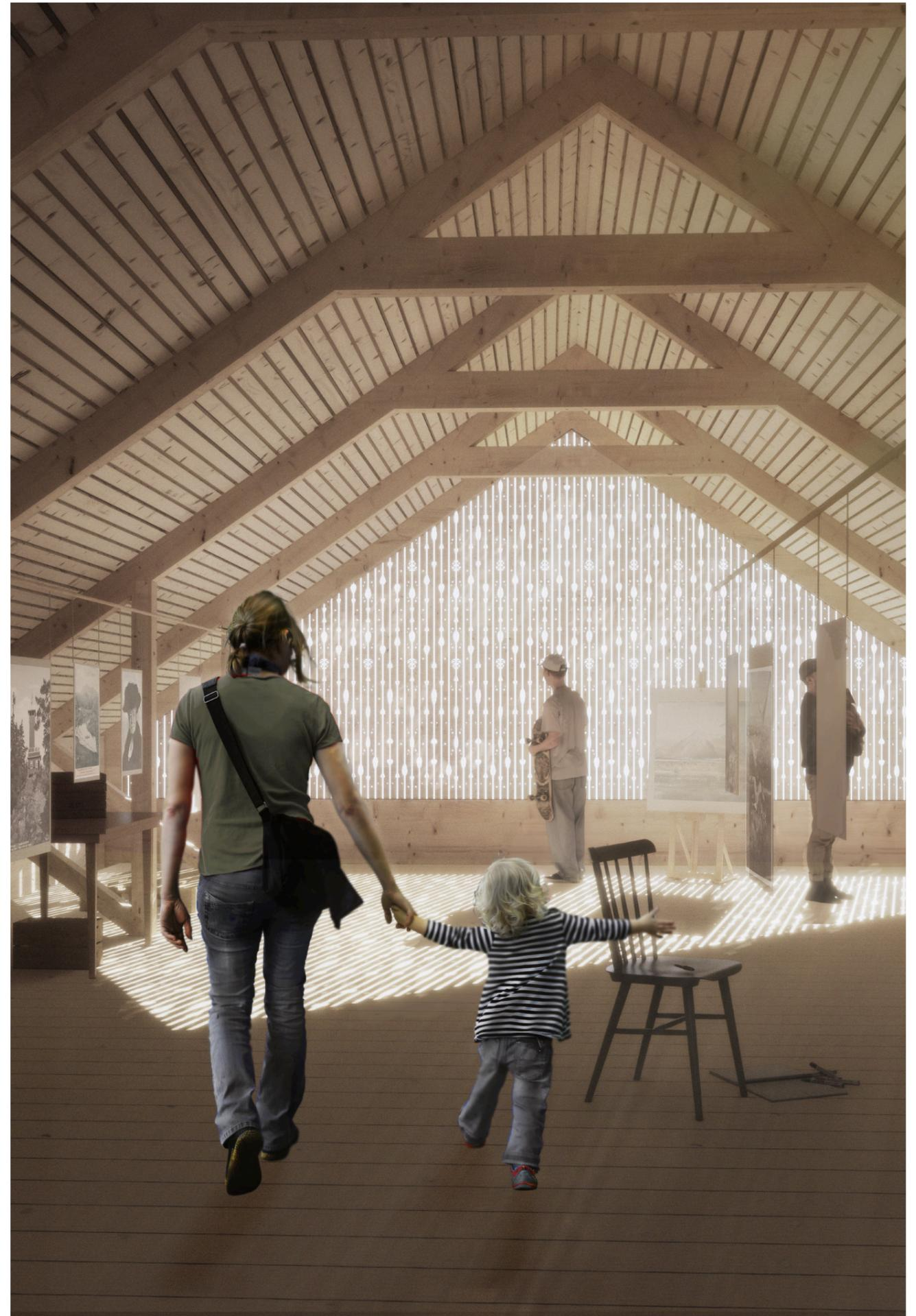
The construction of the roof varies between the building volumes. The north building has partly double ceiling heights and has a roof ridge construction with a central rafter and pillars. In the south buildings, using a wooden framework truss to give an open floor plan for the kitchen without supporting pillars is more suitable.
