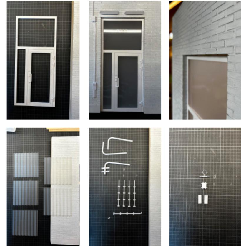
The main part of the scale model details was 3D-printed, glued and painted. Sandpaper cut outs where used to immitate tiles and layed piece by piece.
