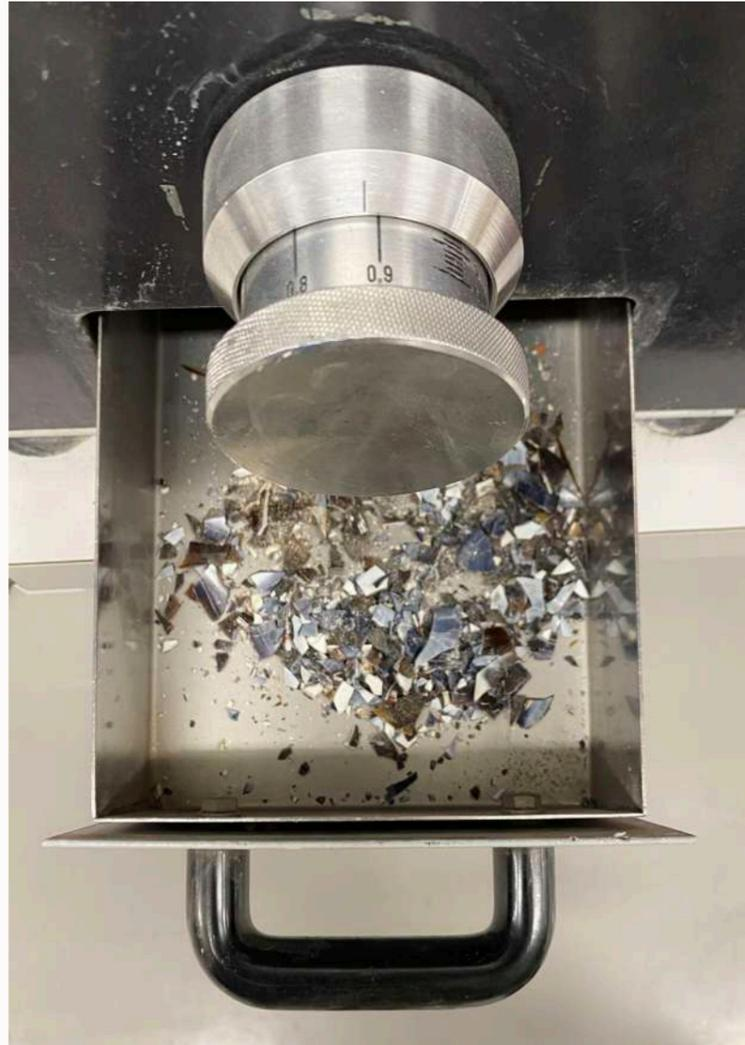
*For shell based aggregate, the machine crushes the shells at different particle sizes depending on purpose*
