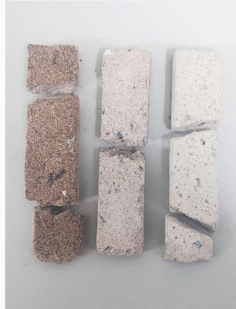
*Different hardened samples based on different recipes. Hardened but fragile.*
