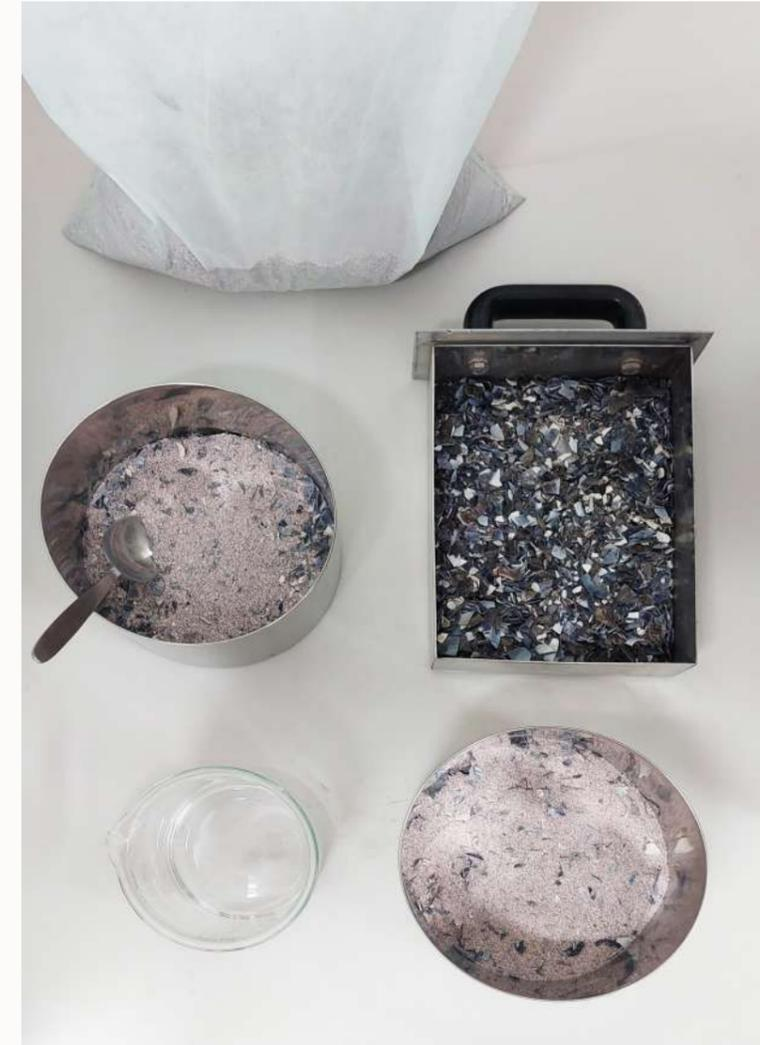
*Different mixtures depending on the recipe is prepared. The mixtures are based on crushed shells, shell-based sand, water and reactive compounds such as lime and volcanic ash or clay.*
