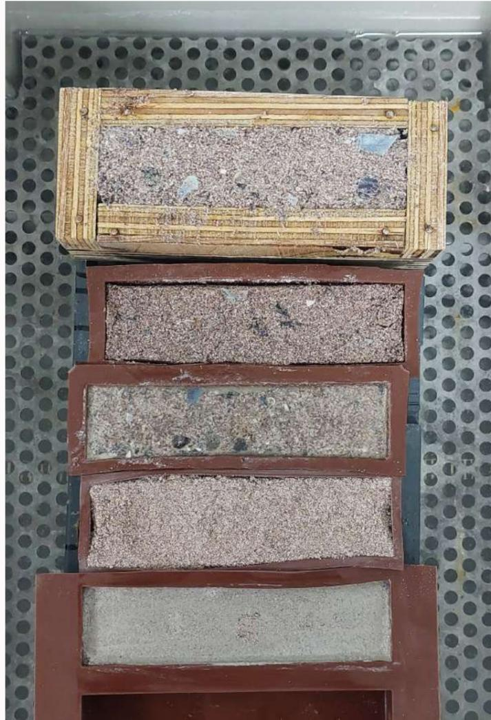
*The mixture needs to harden and here different moulds and mixtures were tried out. The wood one was most successful as it hardened the best. Some mixtures were wetter and needed a longer time to cure.*
