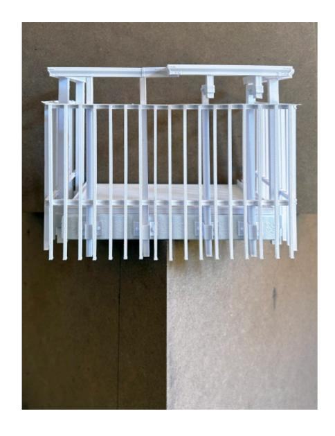
Model assembly - Balcony profiles. PLA Printed
