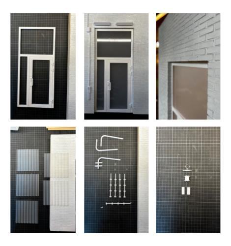
The main part of the scale model details was 3D-printed, glued and painted. Sandpaper cut outs where used to immitate tiles and layed piece by piece.
