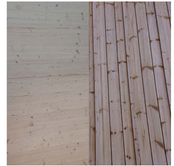
CLT, own photograph from Chalmers. And ThermoWood, own photograph from Titterdamm in Angered.
