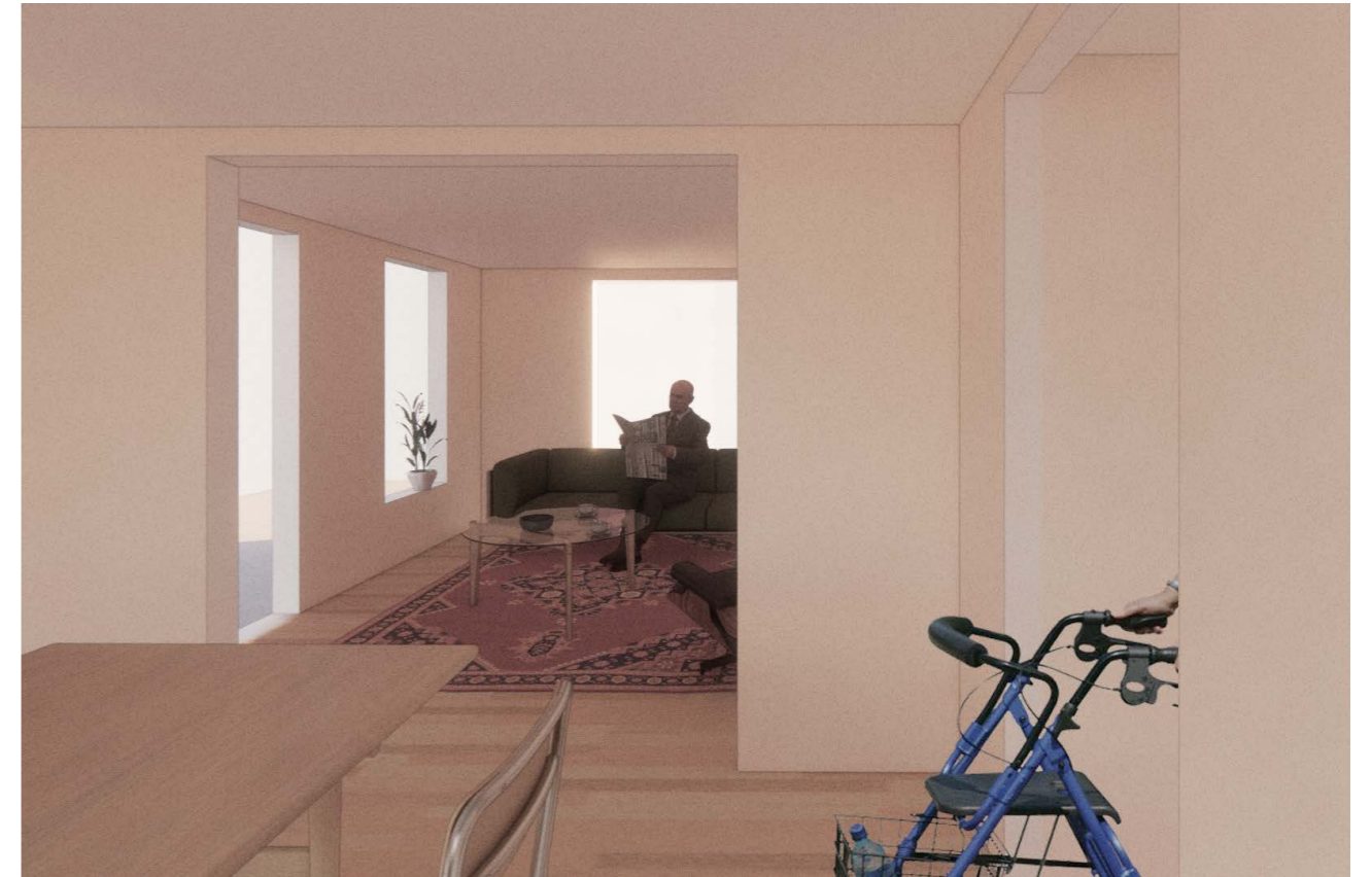
Basement floor - looking from dining space into living room. New openings inside and to the outside makes it possible to move freely in home. Larger windows but kept 45 cm above floor to frame the room and create space to make it more personal.
