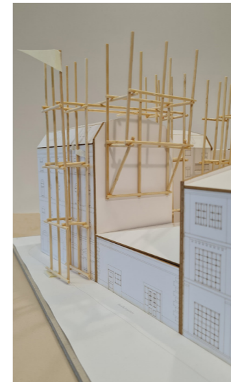
Testing the shape of the structure and how it could be attached to the existing roofs and facades in 1:100 models.
