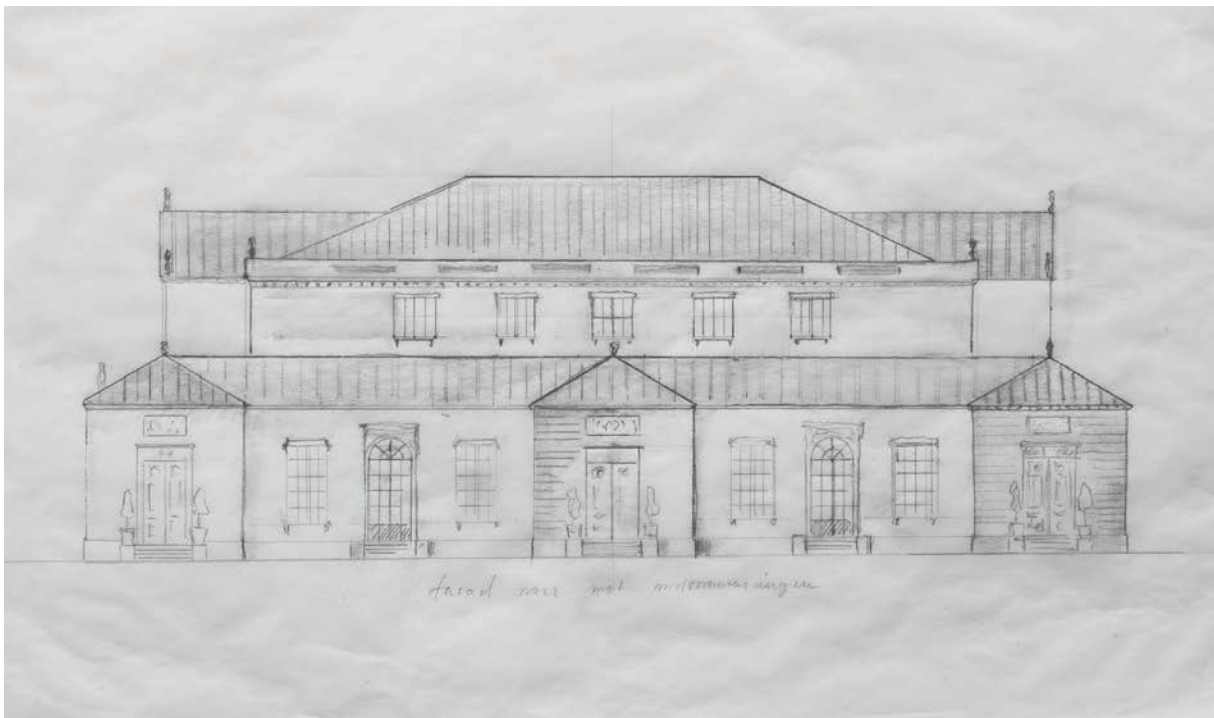
Phase 1. The southern facade With a timbered house body in the center and foyers and back-stage as a collar around the center.
