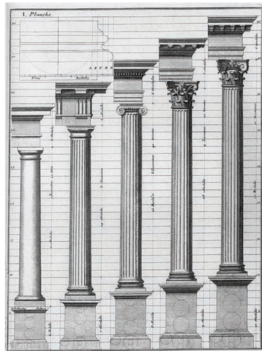
Claude Perrault, France 1676. A copper-plate version of the classical orders where the various parts could be read and memorized.
