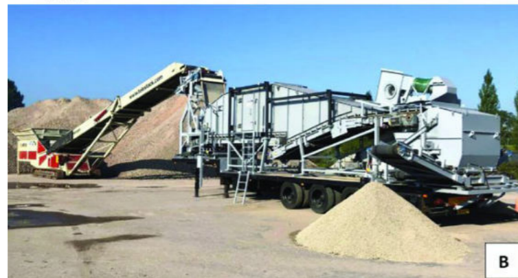
Figure 11 A sketch of ADR working principles (A) and ADR installation on site (B) (Rem et al., 2020)
