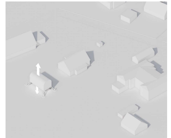
With heavy snowfall and shifting snow, the module is placed on pneumatic legs to elevate structure above.
