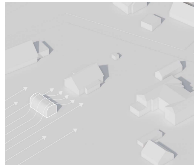
To accommodate for increased frequency and strength of winter storms as well as the precipitation that follows, the module is made aerodynamic
