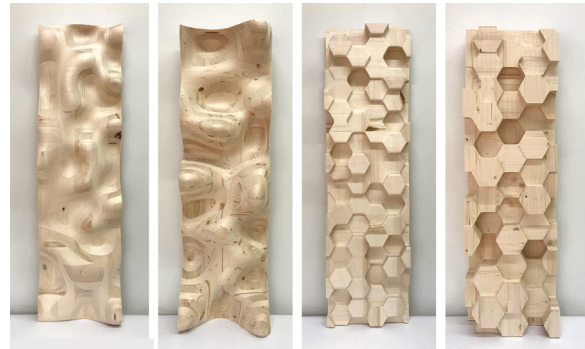
Figure 13, CNC-milled timber prototypes (Peters et al., 2020)
