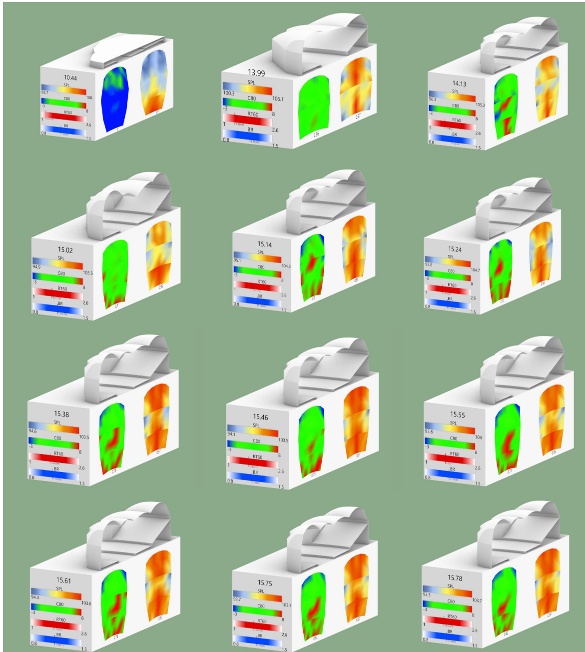
Figure 45, Different solutions from the same iteration process, with each solutions respective fitness value in the top numbers, and acoustical diagrams describing its properties. The program looks for highest possible fitness value.
