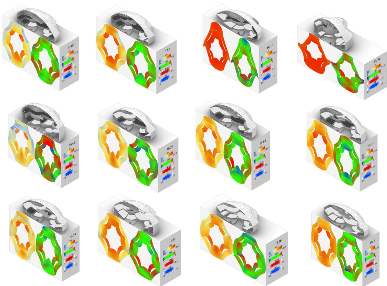
Figure 51, Different solutions from the same iteration process, with each solutions respective fitness value in the top numbers, and acoustical diagrams describing its properties. The program looks for highest possible fitness value.
