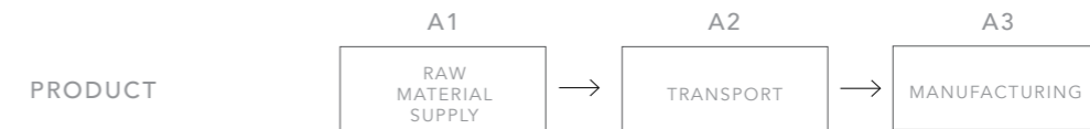
Figure 16, LCA phases A1-A3, shows the all the phases in a life cycle assessment for a material
