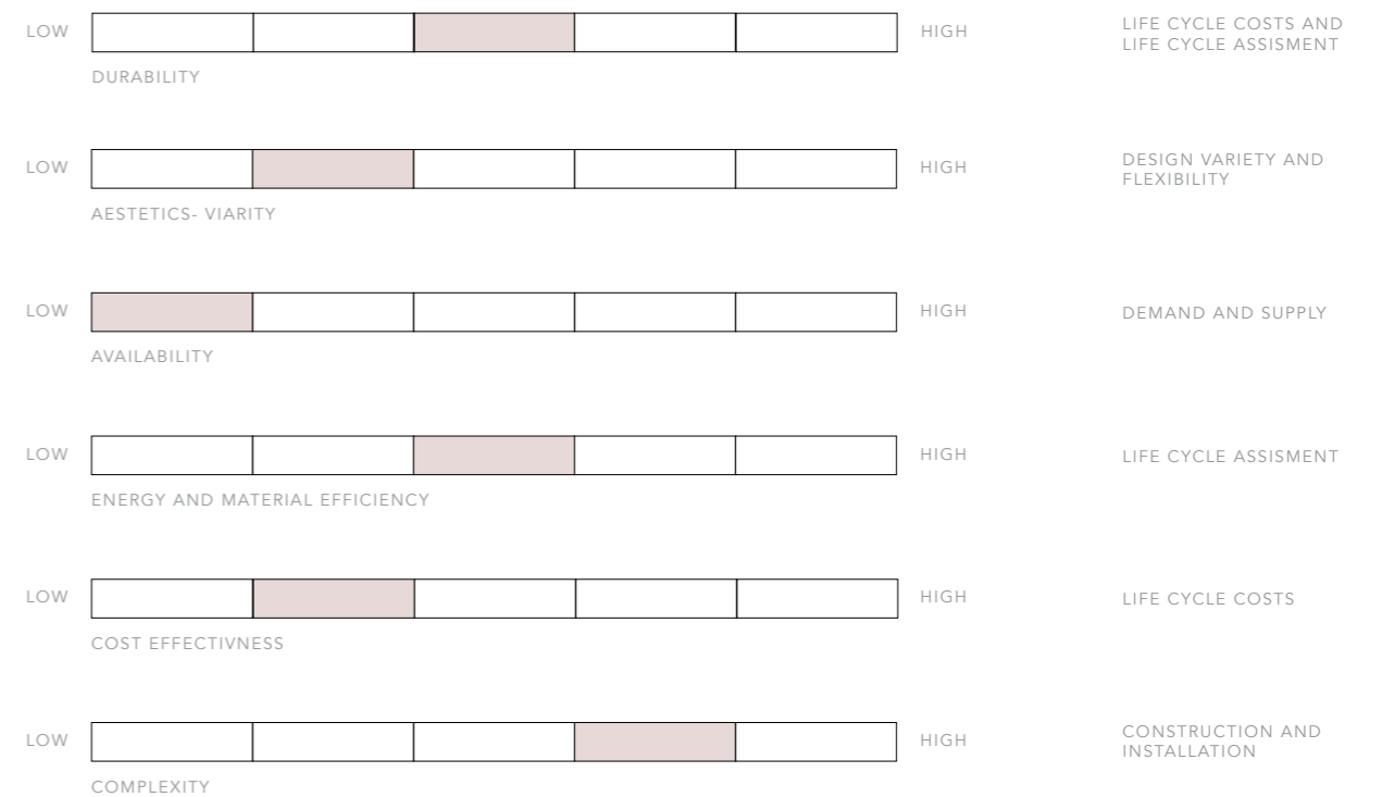
Figure 17, The criteria for material selection, as outlined in the report “Facade Design Stages: Issues and Considerations,” for Case study 2: cut brick element, this serves as a foundation for the discussion on page 67.
