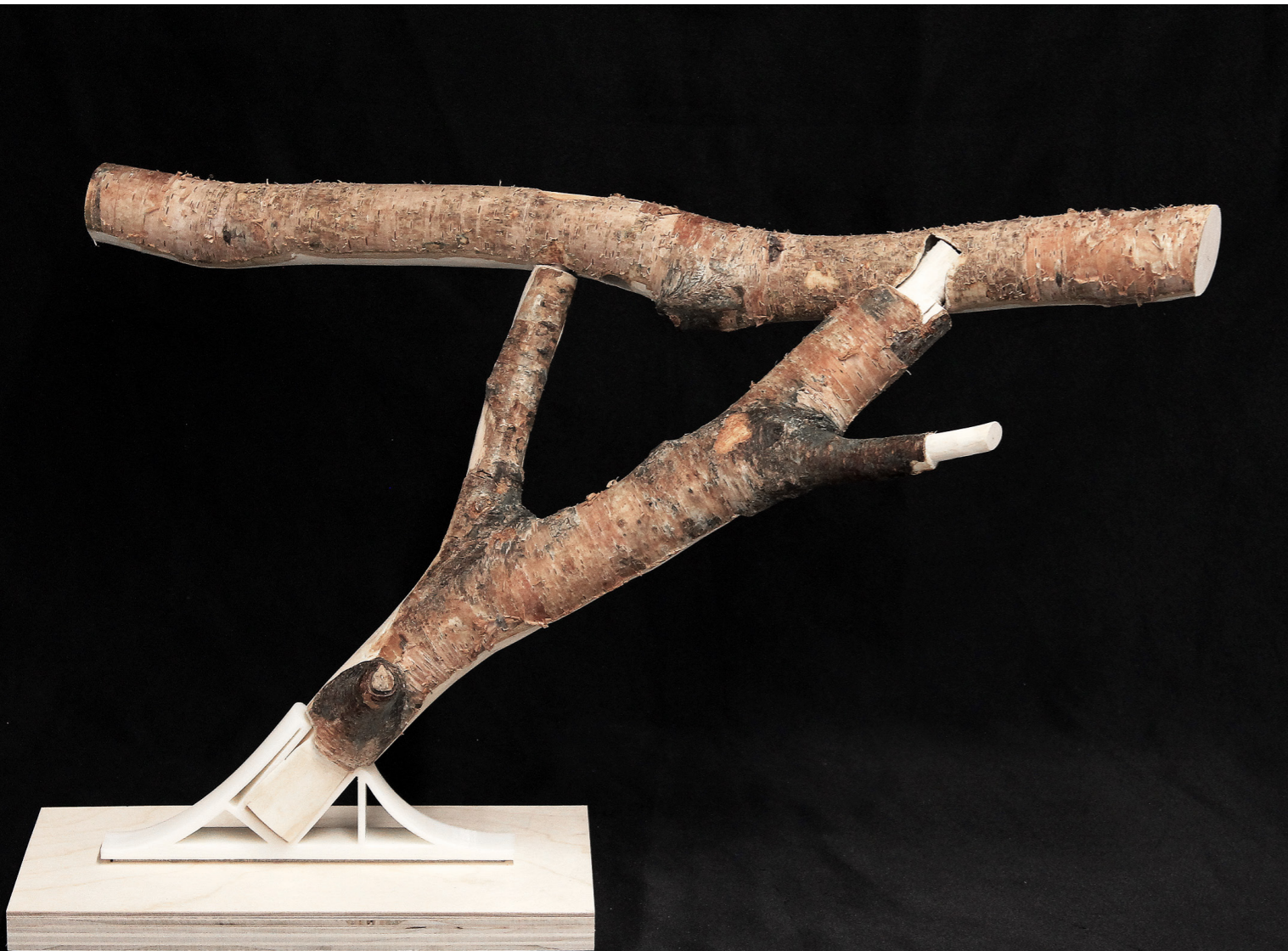
Fig. 65. Top-to-Side connection of a forked piece and a bent piece.
