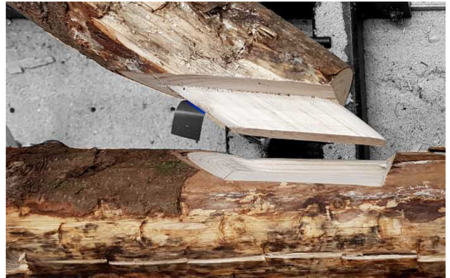
Fig. 17. Tenon-mortise joint from raw wood.
