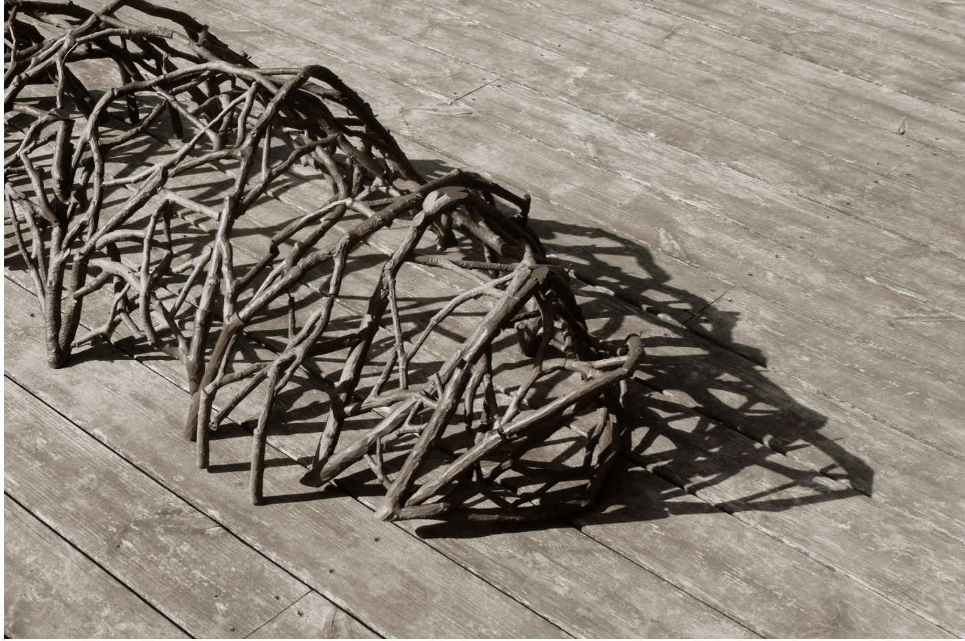
Fig. 51. Prototype 4. Structure Model. Physical raw wood pieces were 3D scanned, and the resulting structure was 3D printed in 1:25 scale.
