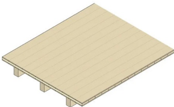
Figure 43d. Drawing of Stora Enso Sylva CLT Rib, the floor slab system used in this transformation. The drawing is a courtesy of Stora Enso
