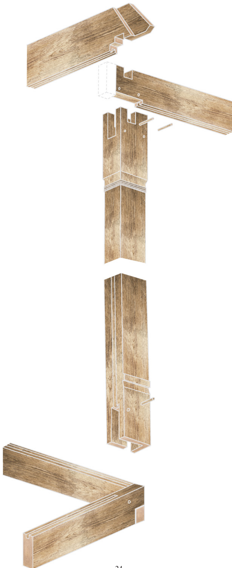
Connection between long sill plate, cross sill plate, corner post, long beam and cross beam.
