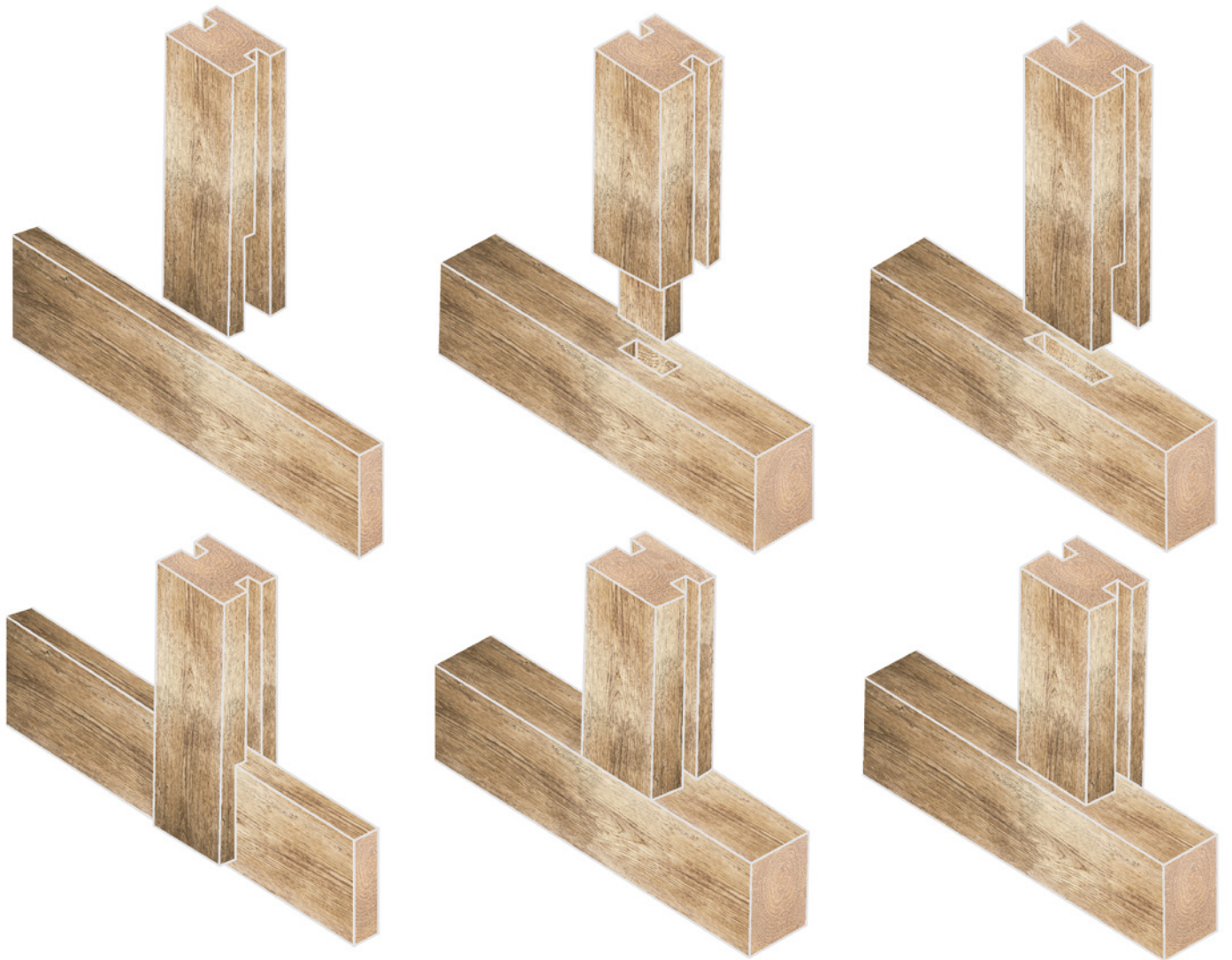
Different connections between sill and post, seen from the inside. In the illustration on the left the timber is oak, in the middle and right the timber is pine.
