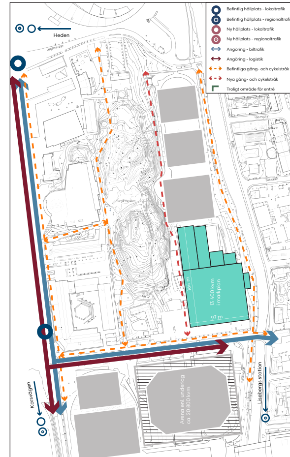
Illustration from the report Fördjupad lokaliseringsstudie av ett nytt centralbad (2018) by Tengbom for Stadsledningskontoret Göteborg. The diagram shows the present day conditions of the site, with schematic projections of the new public bath in teal and other planned development in gray.
