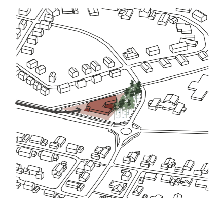
Figure 45: The entrance are placed towards Karlskrona city center and the bus stop and the common outdoor area are placed towards the forest at a calm and enclosed place.
